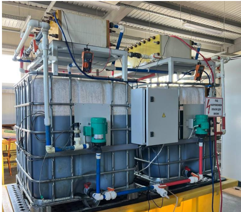
Figure 2. Photo of a UPS with 2 stacks of vanadium redox flow battery.
