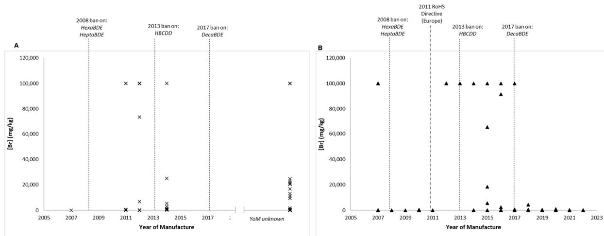
**Figure 3.** The variation in bromine concentration determined via h-XRF according to the YoM of the equipment. (A) Br concentration determined for items in Company 1 vs. Year of Manufacture. (B) Br concentration determined for items in Company 2 vs. Year of Manufacture.
