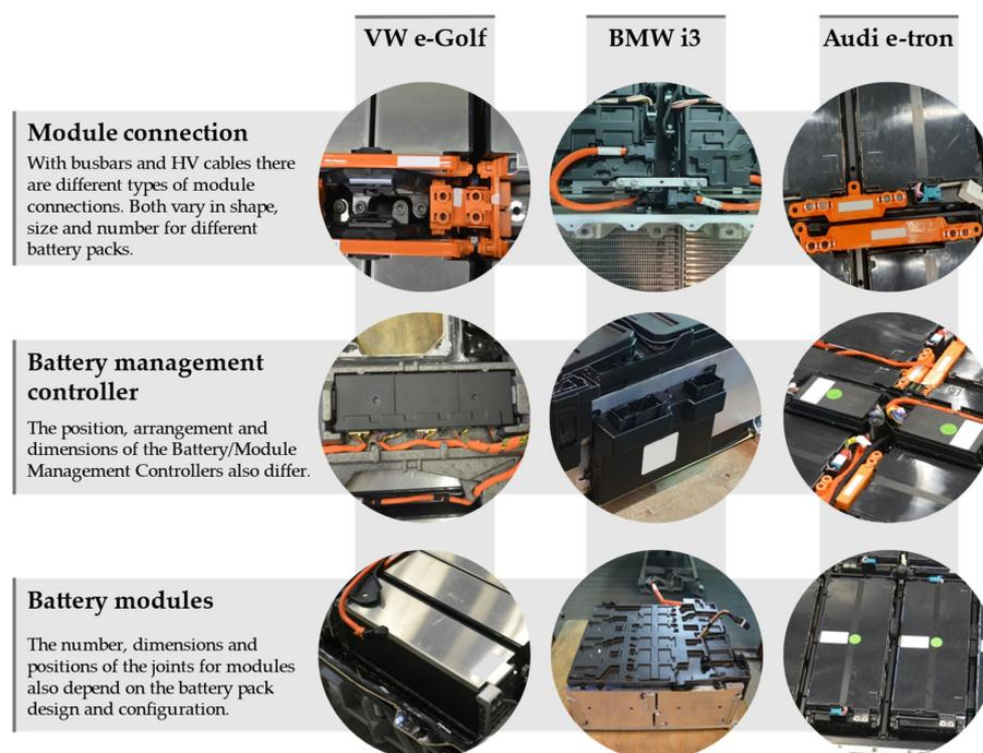
**Figure 3.** Differences in the design of functionally equivalent battery components for three different vehicle models.
