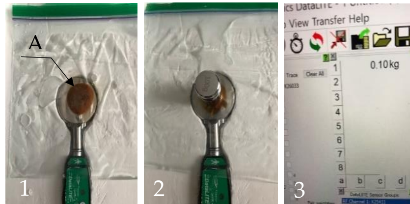
Figure 2. Effect on pressure transmission via a solid plug isolating the walls of the bag from the surrounding water. (1) Bag and the plug (A), made of caramelized sugar with water surrounding it; (2) placement of a weight of 0.1 kg above the plug; (3) load of 0.1 kg registered on computer screen.
