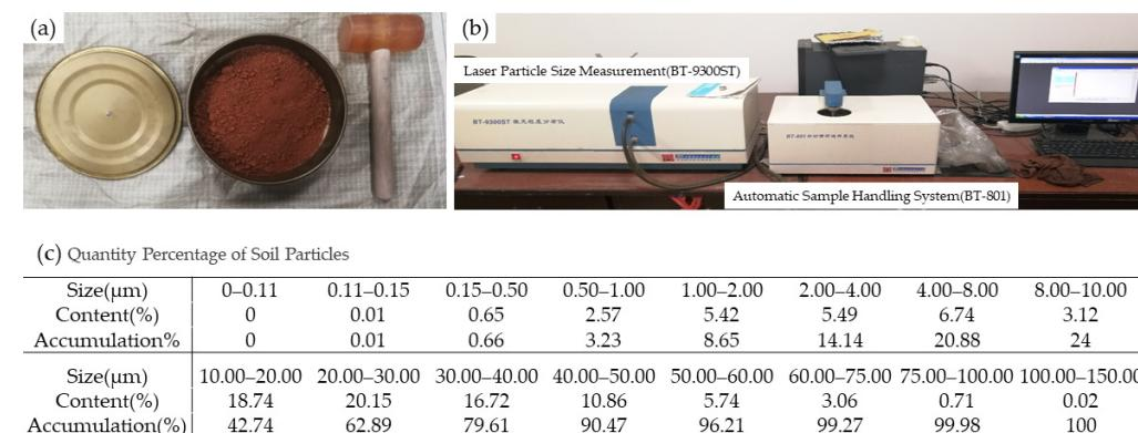
**Figure 5.** (a) Soil sieving; (b) soil analyzing; (c) results of soil analyzing.
