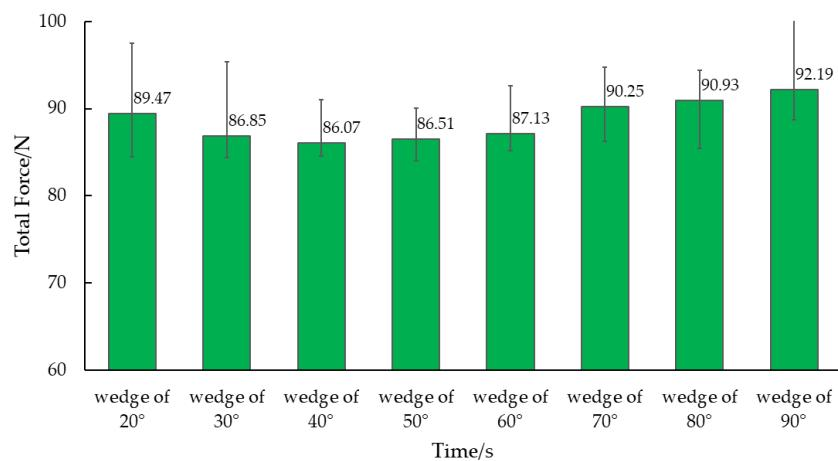
**Figure 10.** Simulate motion resistance of different wedges.
