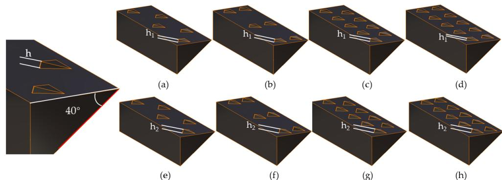
**Figure 11.** Non-smooth surface wedges with different microstructures: (a) wedge of low-tail sparse staggered distribution; (b) wedge of low-tail sparse parallel distribution; (c) wedge of low-tail dense staggered distribution; (d) wedge of low-tail dense parallel distribution; (e) wedge of high-tail sparse staggered distribution; (f) wedge of high-tail sparse parallel distribution; (g) wedge of high-tail dense staggered distribution; (h) wedge of high-tail dense parallel distribution.
