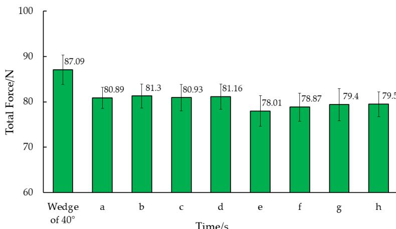
a wedge of low-tail sparse staggered distribution; b wedge of low-tail sparse parallel distribution; c wedge of low-tail dense staggered distribution; d wedge of low-tail dense parallel distribution; e wedge of high-tail sparse staggered distribution; f wedge of high-tail sparse parallel distribution; g wedge of high-tail dense staggered distribution; h wedge of high-tail dense parallel distribution.
