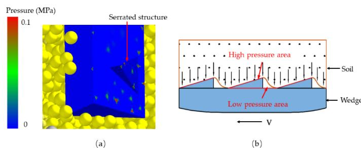
**Figure 14.** (a) The stress distribution on the surface of the wedge; (b) the contact model of soil and soil-engaging components.
