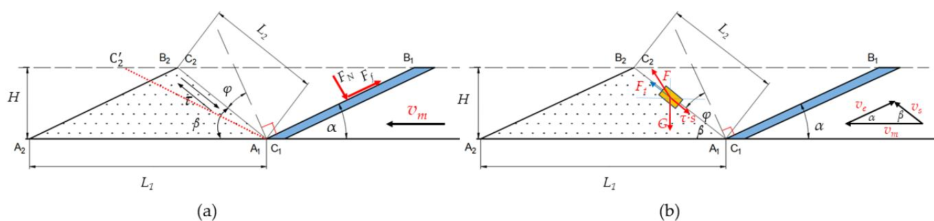
**Figure 13.** (a) Motion state of the wedge. (b) Motion state of the soil particle.
