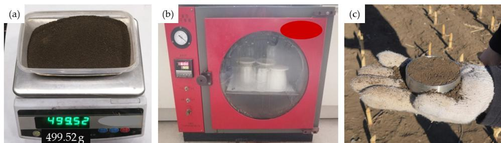
**Figure 4.** (a) Soil weighing; (b) soil drying; (c) soil sampling.
