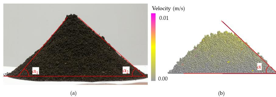
**Figure 7.** (a) Measurement of soil repose angle; (b) simulation of soil repose angle.
