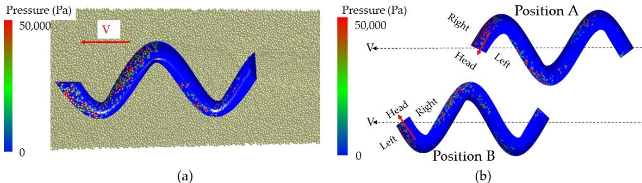
**Figure 8.** (a) EDEM simulation of the movement of sandfish model in soil; (b) states at different times of sandfish model.
