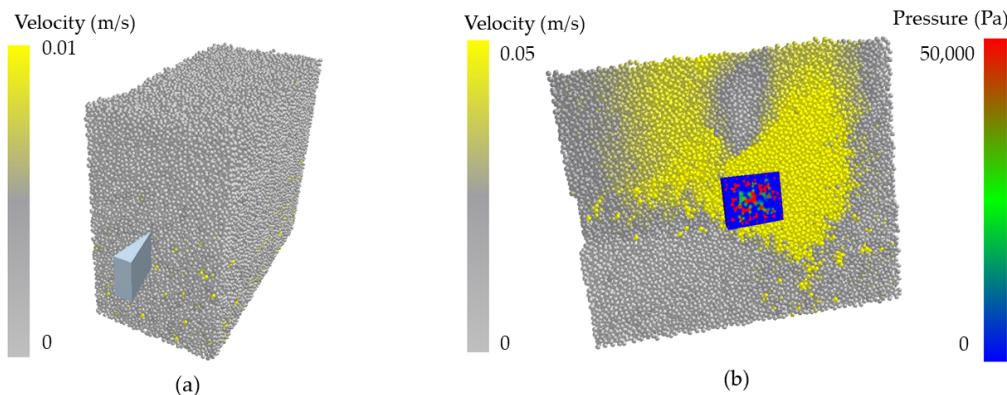
**Figure 9.** (a) Soil particle generation and wedge model import; (b) the state of wedges at a certain moment.
