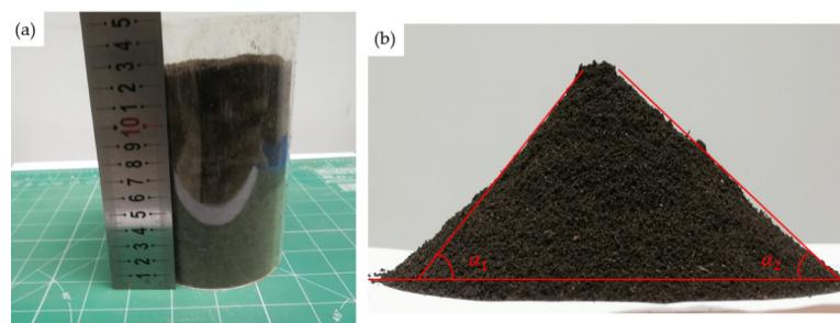
**Figure 6.** (a) Preparation of soil repose angle measurement; (b) process of soil repose angle measurement.
