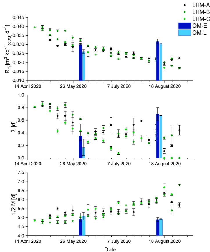
**Figure 6.** Kinetic parameters  $R_m$  ( $\text{m}^3 \text{kg}^{-1} (\text{oDM}) \text{d}^{-1}$ ),  $\lambda$  (d),  $\frac{1}{2} M$  (d), using the modified Gompertz function of three lowland hay meadows (LHMs) characterised by different conservation statuses (A = excellent, B = good, and C = average) over the vegetation period and of orchard meadows in two different regions (E = Eningen and L = Lichtenstein) at two harvest dates at Swabian Jura.
