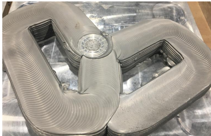
Figure 4. Onion skin observed on the top surface of a deposition.
