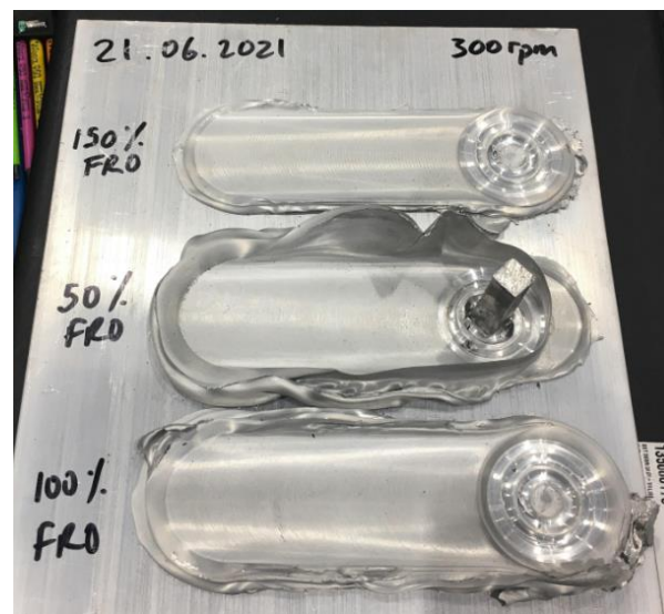
Figure 5. Influences of feed rate override (FRO) on flash formation during AA6061 AFSD process under constant rotational speed.
