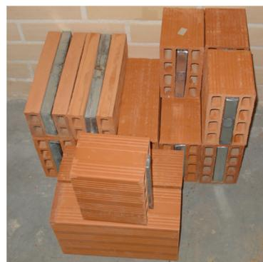
**Figure 14.** Clay bricks and PCM macro-capsules integration, Silva et al. [133] (reproduced with permission from Elsevier).
