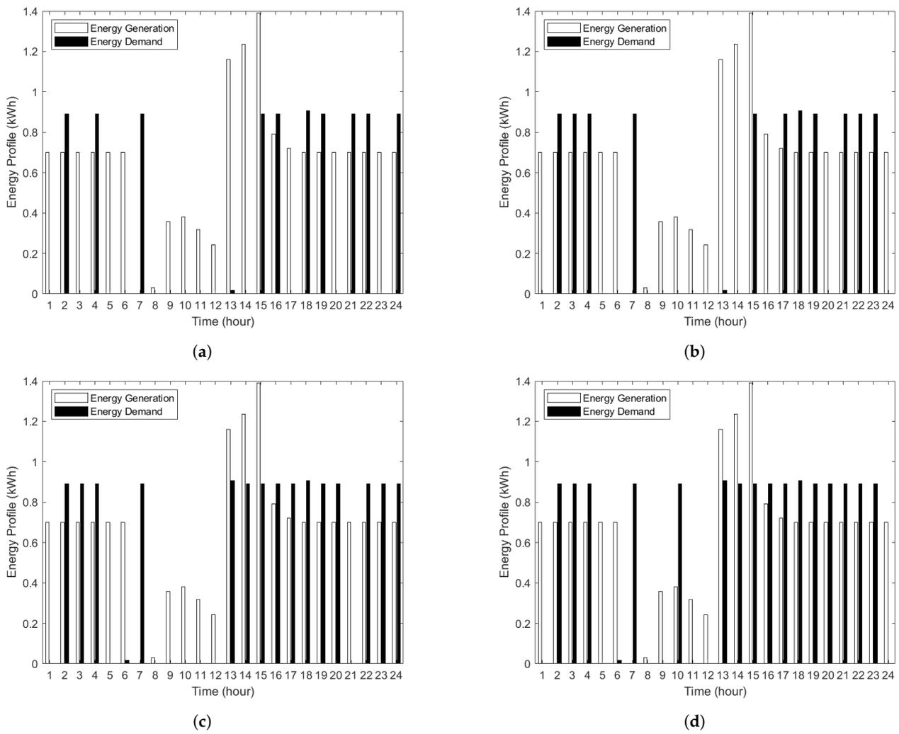
**Figure 5.** Energy profiles of four different PFAs in winter: (a) SPFA/S, (b) SPFA/GS, (c) MPFA/SG, and (d) MPFA/MG.
