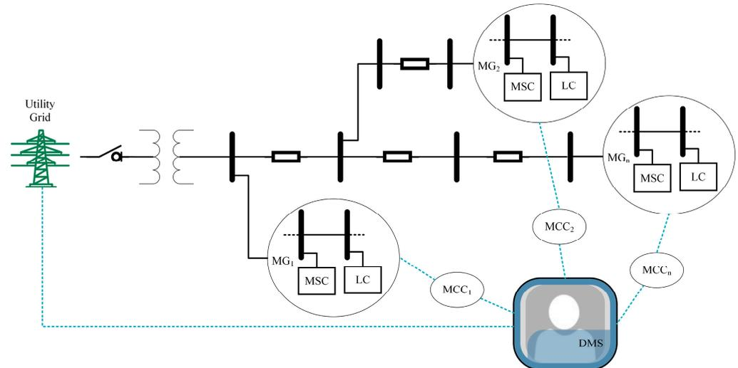
Figure 9. MG control diagram.
