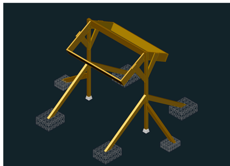
Figure 2. Inverse Y ballast system.
