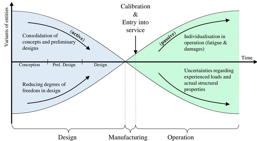
**Figure 6.** Variety of entities in the Digital Twin in the design and operation phases.
