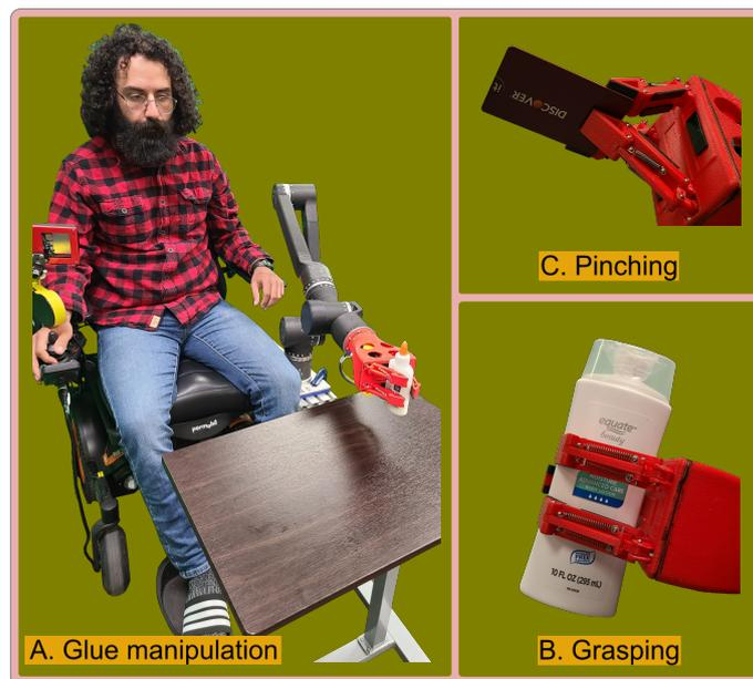
Figure 2. The figure captures the gripper performing three distinct functions: (A) Glue manipulation, showing the gripper’s fine motor control and dexterity. (B) Grasping, illustrating the gripper’s ability to hold larger objects securely. (C) Pinching capability, where the gripper adeptly handles slim objects like a credit card, showcasing the precision and versatility.
