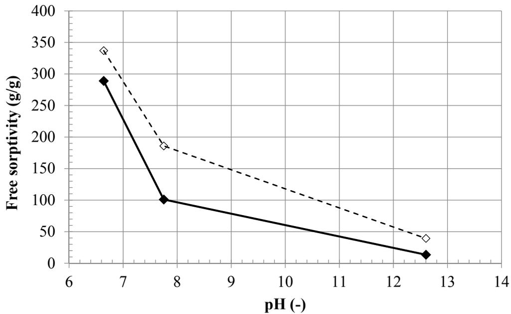
Figure 4. Absorption capacity (free sorptivity) of SAP<sub>CT</sub> (bold line) and SAP<sub>PT</sub> (dashed line).
