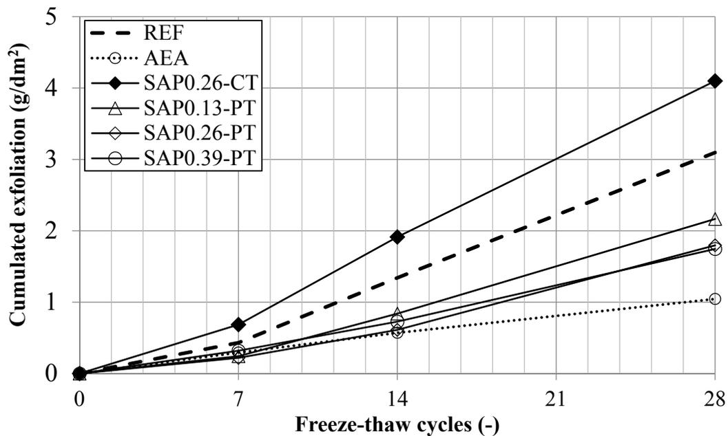
Figure 7. Cumulated exfoliation of the different mixes after 28 cycles (FT1 method).
