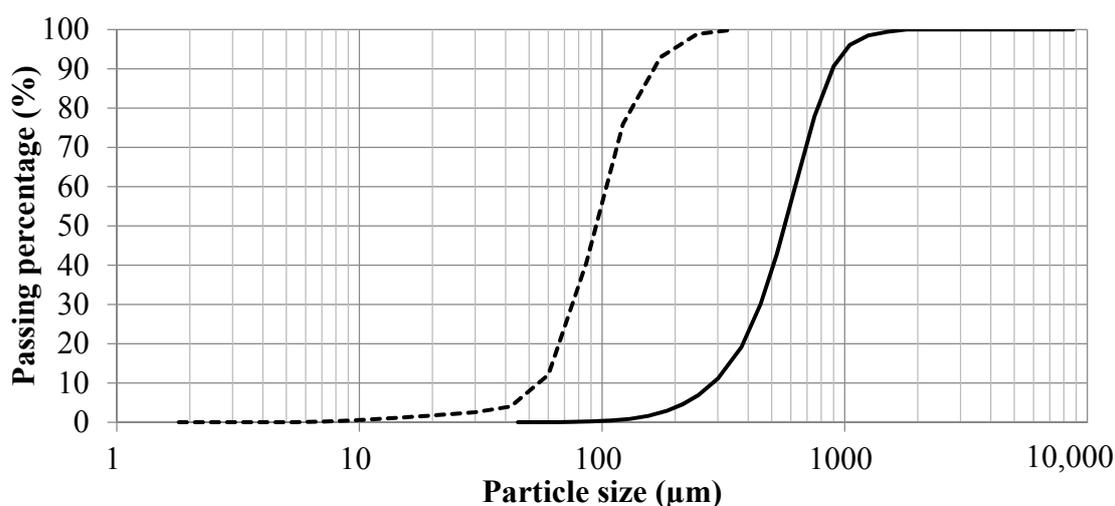
Figure 3. Particle size distribution of SAP<sub>CT</sub> (bold line) and SAP<sub>PT</sub> (dashed line).
