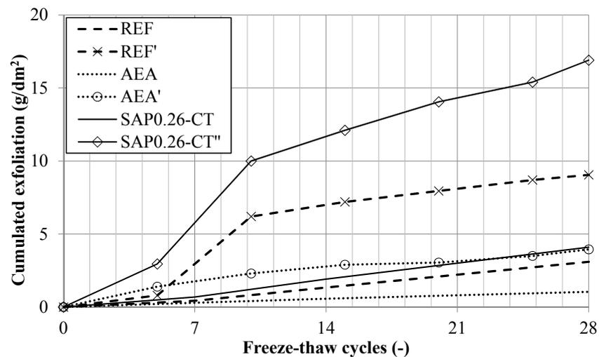
**Figure 8.** Cumulated exfoliation of the different concrete mixes with AEA and SAP<sub>CT</sub> after 28 cycles (FT1 vs. FT2 method).
