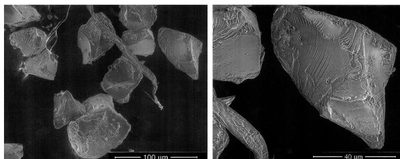
**Figure 2.** SEM images of SAP<sub>PT</sub> particles.
