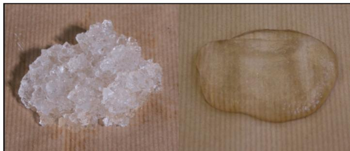
**Figure 1.** Visualization of superabsorbent polymers (SAPs): SAP<sub>CT</sub> (left) and SAP<sub>PT</sub> (right) containing absorbed water.
