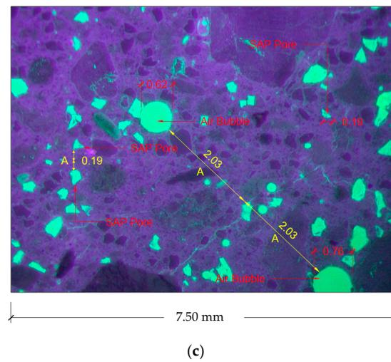
**Figure 9.** Images of microscopic analysis (petrography on thin sections) of (a) REF, (b) SAP0.26<sub>CT</sub> and (c) SAP0.26<sub>PT</sub>.
