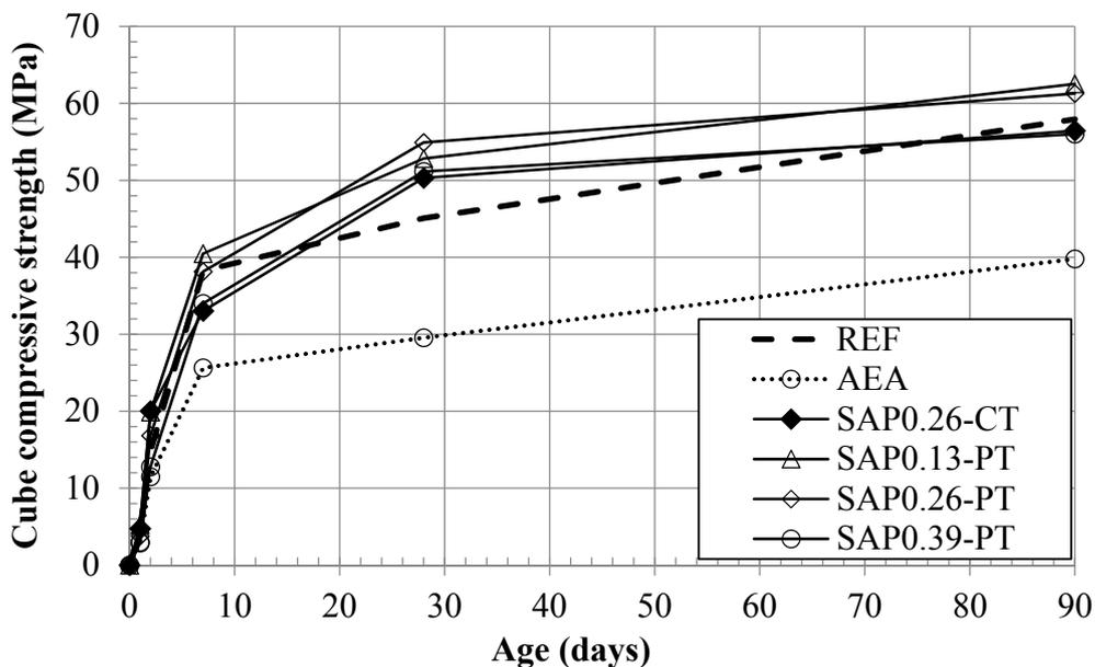
Figure 6. Cube compressive strength development of the different concrete mixes between ages of 1 day and 90 days.
