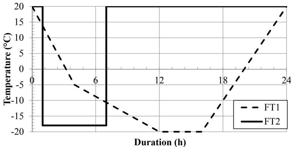
Figure 5. Freeze–thaw temperature cycles of the CEN/TS 12390-9 (FT1) and the ISO/DIS 4846-2 (FT2).
