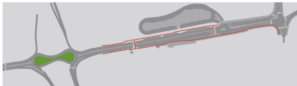
**Figure 6.** Future network—Scenario 1.1 (red: bicycle network; dark grey: traffic network; light grey: pavement) (Figure extracted from the PTV VISSIM simulation software [9]).
