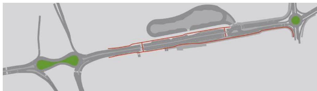
**Figure 7.** Future network—Scenario 1.3 (red: bicycle network; dark grey: traffic network; light grey: pavement) (Figure extracted from the PTV VISSIM simulation software [9]).
