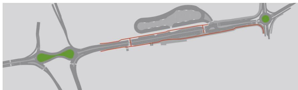
**Figure 8.** Future network—Scenario 1.4 (red: bicycle network; dark grey: traffic network; light grey: pavement) (Figure extracted from the PTV VISSIM simulation software [9]).
