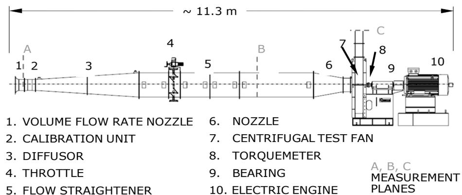
Figure 2. Pipe test rig according to ISO 5801:2018 with high-pressure centrifugal fan.
