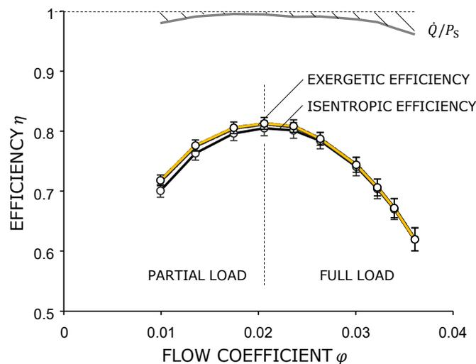
Figure 4. Exergetic efficiency compared to isentropic efficiency. The calculated power loss due to heat dissipation to the environment is hatched.
