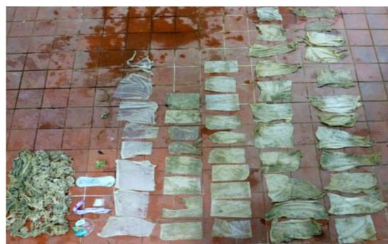
**Figure 1.** Constituents of pump blockage [3].
