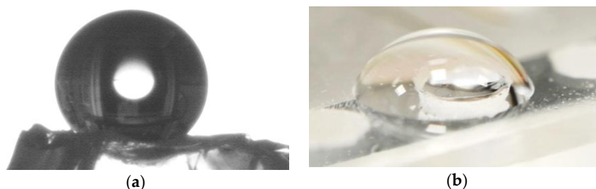
Figure 5. (a) Water droplet on the surface of a silica aerogel block. The contact angle is 136°; (b) Water droplet on one of the holes containing the aerogel. The water does not flow through the hole with the gel despite its high porosity of 85% in contrast to a second setup without aerogel.
