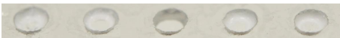
Figure 3. Microchip made of 500 \mu\text{m} thick borosilicate glass with holes of 1.2 mm diameter. Four holes were filled.
