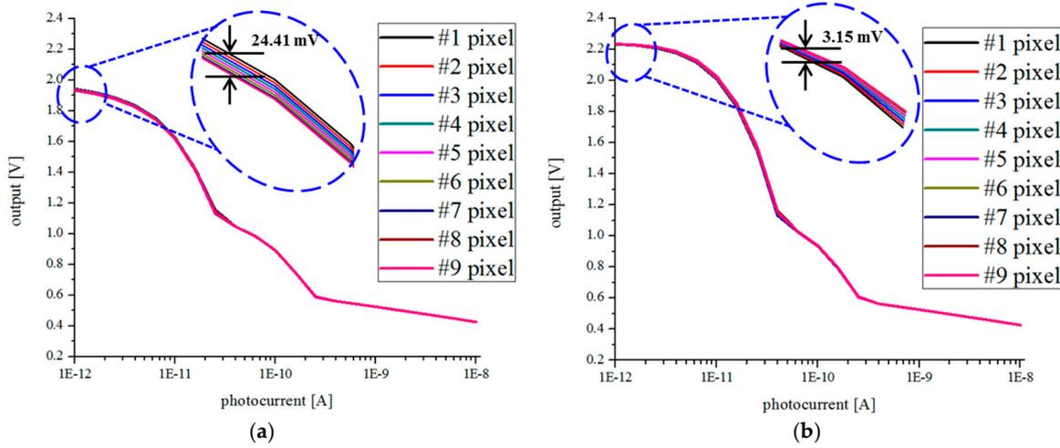
**Figure 2.** Simulation results of output curves according to the reset method; (a) conventional linear-logarithmic pixel and (b) proposed linear-logarithmic pixel.
