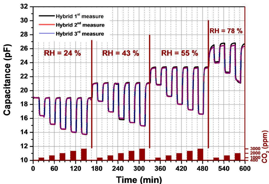
**Figure 2.** Capacitance response versus time of amine functionalized silica nanoparticles based CO<sub>2</sub> sensor. Capacitance change recorded under different CO<sub>2</sub> concentrations and relative humidity levels.
