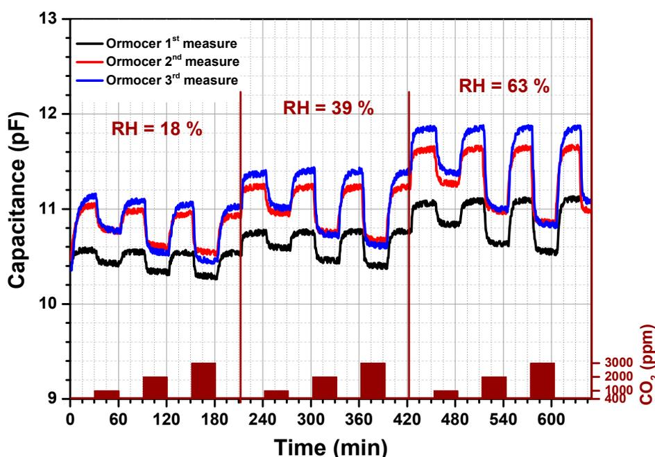
**Figure 1.** Capacitance response versus time of Ormocer based CO<sub>2</sub> sensor. Capacitance change recorded under different CO<sub>2</sub> concentrations and relative humidity levels.
