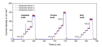
**Figure 2.** Transient raw signal (blank subtracted) from 3 glutamate sensors upon addition of different types of food samples (instant broth).
