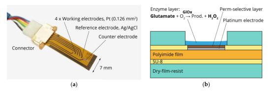
**Figure 1.** (a) Photograph of sensor platform including platinum working and counter electrodes and silver/silver chloride reference electrode; (b) Schematic cross-section of thin-film/laminate technology and sensor principle. Glutamate is converted by glutamate oxidase (GlOx) into hydrogen peroxide, which is oxidized at the platinum electrode.
