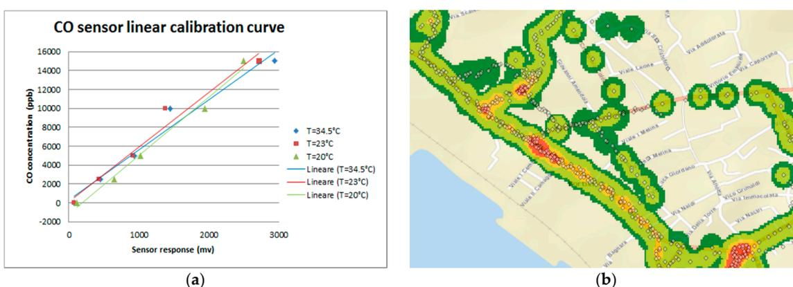
**Figure 4.** (a) CO sensor linear calibration curves at different temperatures; (b) time averaged pollution maps generated by preliminary experiments conducted in the city of Portici (NA), Italy. Red areas indicates significant pollution in areas usually affected by high car traffic.
