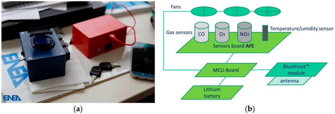
**Figure 1.** (a) Two MONICA 2.0 system prototypes, one of which featuring a bike mounting device and (b) the MONICA 2.0 node architectural scheme.
