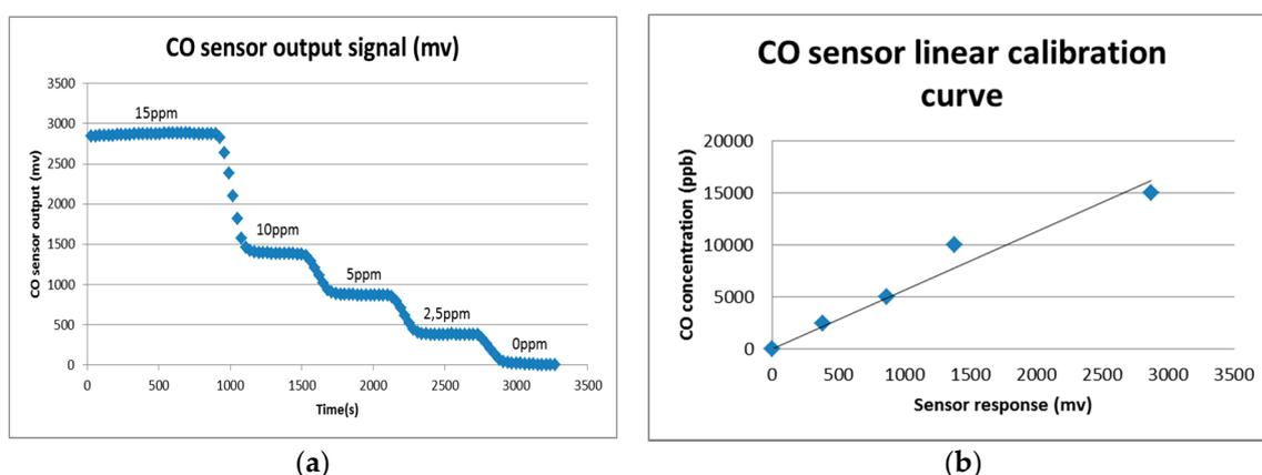
**Figure 3.** (a) CO sensor response during in lab univariate calibration recordings and the corresponding linear calibration curve.
