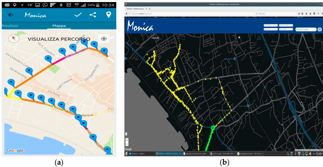
**Figure 2.** (a) Android App activity showing the colour coded route during a mobility session and (b) an example of the web based pollution map built with simulated data.
