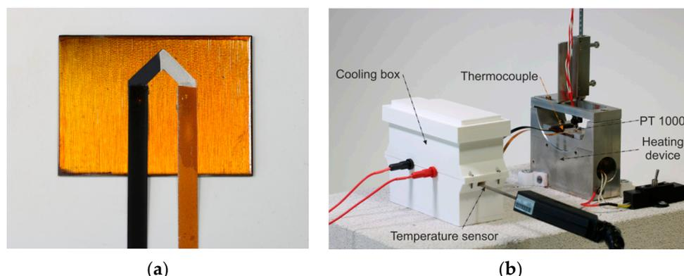
**Figure 2.** (a) spray processed thermocouple on metal substrate with polyimide connections before top coating; (b) Thermocouple test rig consisting of the heating device, a PT 1000 (for measuring the thermocouple junction temperature), a cooling box with aluminum blocks (for keeping the connection temperature constant) and a temperature sensor to measure the connection temperature.
