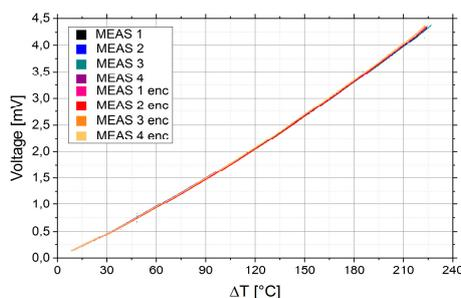
**Figure 3.** Graph of the recorded voltage over the temperature difference between junction and the connection for the uncoated (abbreviated with MEAS 1–4) and top coated (abbreviated with MEAS 1–4 enc) thermocouple.
