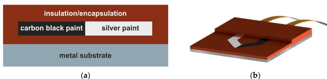
**Figure 1.** (a) Schematic architecture of the embedded thermocouple. The metal substrate is coated with a polyamide-imide insulation layer on which the thermocouple (consisting of the carbon black paint and the silver paint) is processed. The top layer is made out of the same material as the insulation (b) schematic representation of the embedded thermocouple. The polyimide connections (depicted in orange) are coated with the carbon black or the silver paint.
