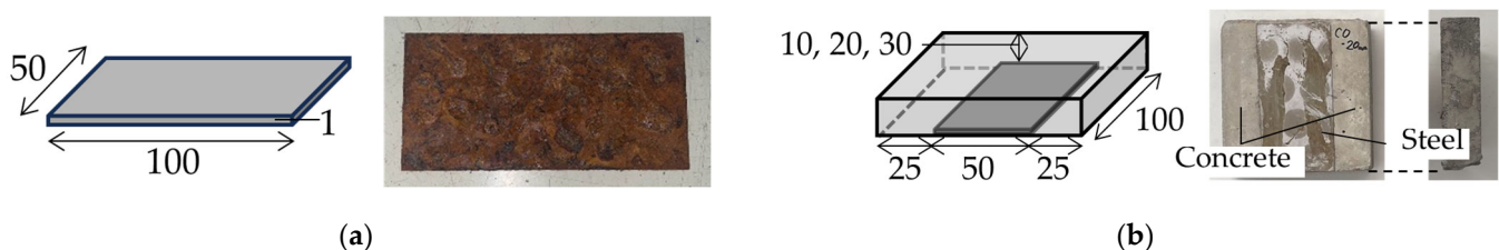
Figure 2. An image of specimens: (a) Steel specimens. (b) Steel-embedded specimens (unit: mm).
