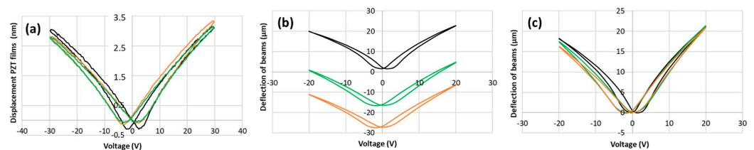
**Figure 3.** (a) Displacement of PZT films, and deflection curves of 500 μm long PZT beams (b) without and (c) with normalization of the deflection. For all 3 figures: PZT deposited (—), PZT reported via Au bonding (—), and PZT reported via SiO<sub>2</sub> bonding (—).
