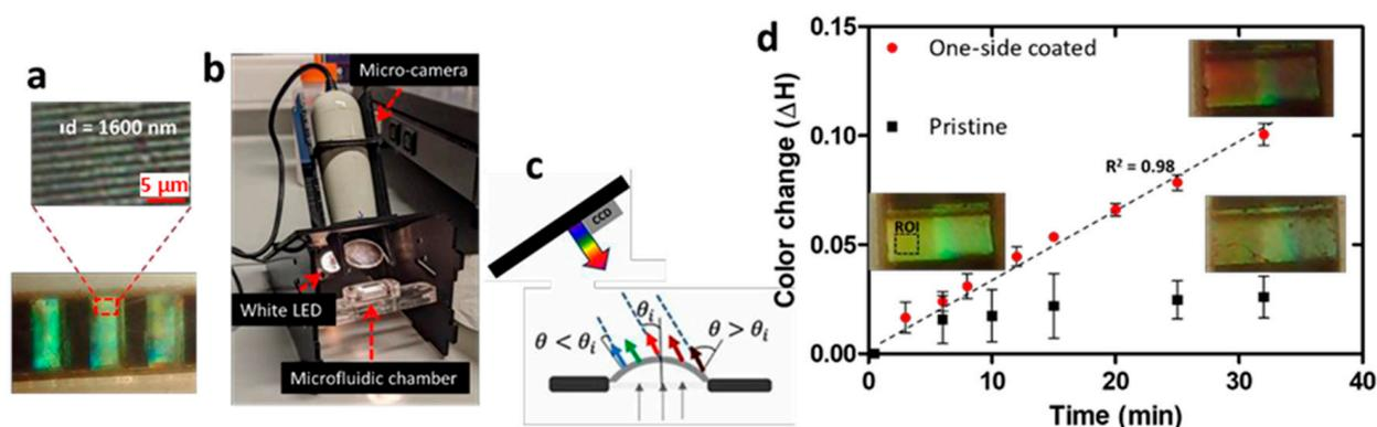
**Figure 1.** (a) Image of the OSTE optomechanical bridges and optical microscopy image ( $50\times$ ) of the periodical surface structure. (b) Color imaging setup. (c) Working principle of the sensors. (d) Color changes during the reduction of MTT for pristine sensors and sensors coated on one side with PEI.
