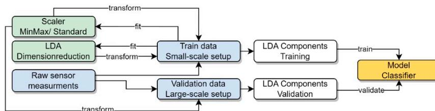
**Figure 1.** Data pipeline; blue: data sets, green: training data-based transformation parameters, white: derived transformation parameters for new feature space, yellow: classification model.
