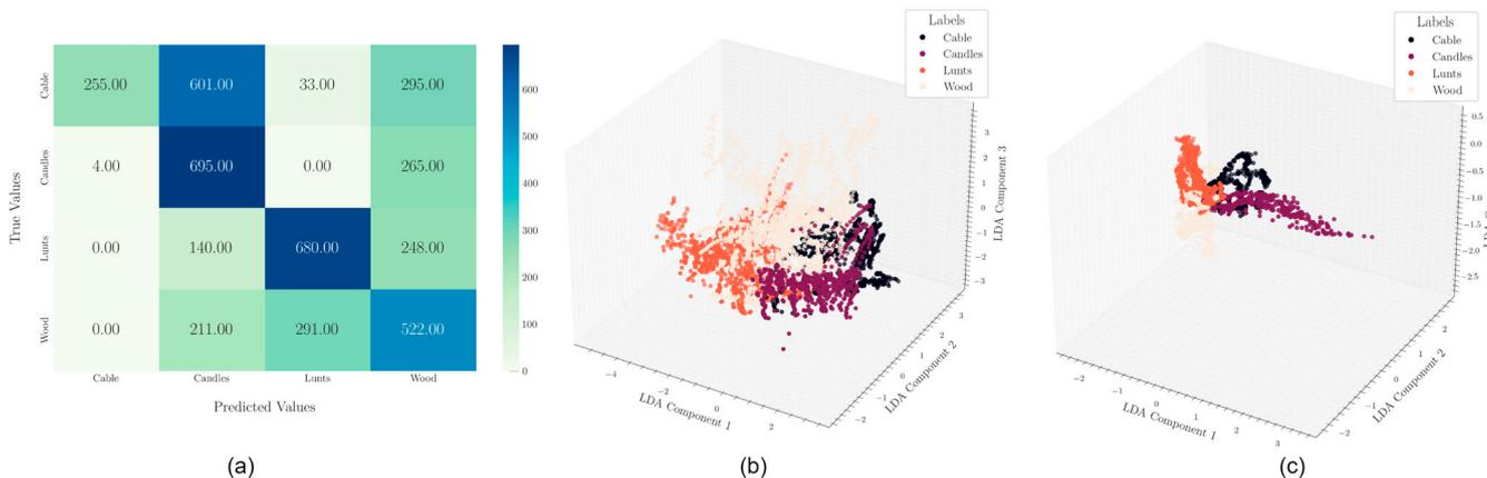
**Figure 2.** (a) Confusion matrix of SVM classifier distinguishing between 4 types of fire materials, (b) class separation of the training dataset using three LDA components, and (c) class separation of the validation data in the same feature space.
