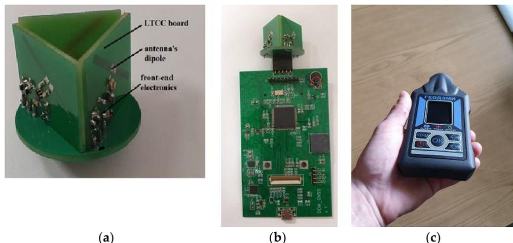
**Figure 1.** (a) Photograph of antenna unit; (b) antenna unit on electronic board of mobile GEO-DOSE dosimeter; (c) mobile dosimeter.
