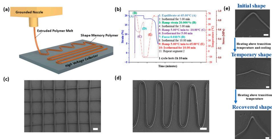
**Figure 1.** (a) Schematic of the MEW process; (b) DMA data obtained and process steps used; (c) grid-like structure; (d) sinusoid structure obtained for SMP; (e) shape memory effect in printed fibers. Scale bars: 200  $\mu\text{m}$ .
