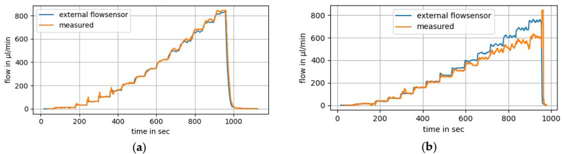
**Figure 2.** Comparison of the measured flow rate with our hot wire sensor and the measured flow rate of an external sensor (a) directly after calibration and (b) two days after calibration.
