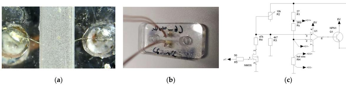
**Figure 1.** (a) Etched Wollaston wire in the channel soldered to copper wires at each end; (b) fabricated flow sensor; (c) circuit to switch between two temperature levels.
