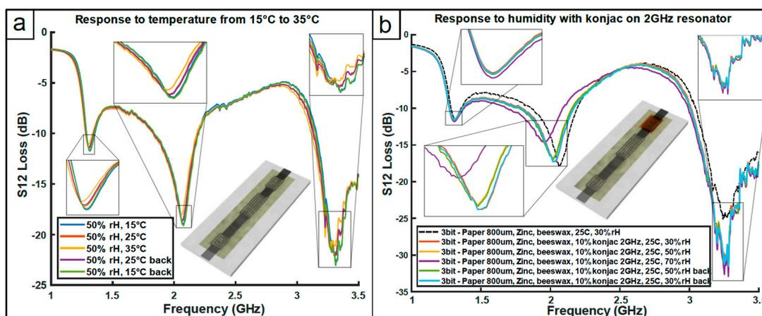
**Figure 1.** S12 signal of the ecoresorbable microstrip platform (noise at 3 GHz due to climatic chamber operation). (a) S12 temperature response of the multi-resonating structure cycling from 15  $^{\circ}\text{C}$  to 35  $^{\circ}\text{C}$  and down, with device schematic; (b) S12 relative humidity response of the multi-resonating structure cycling from 30% RH to 70% RH and down, with device schematic.
