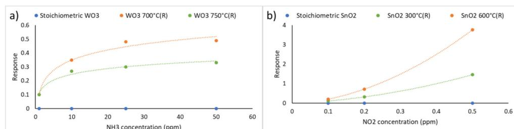
**Figure 1.** (a) Sensing responses, at a working temperature of 70 °C, of (a) stoichiometric and reduced (R)  $WO_3$  powders vs.  $NH_3$  and (b) stoichiometric and reduced (R)  $SnO_2$  powders vs.  $NO_2$ .
