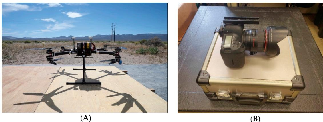
**Figure 2.** Uncrewed aerial system (UAS) equipment used in this workflow. (A) Gryphon UAS used during flight missions. (B) Canon EOS 5D Mark IV DSLR camera, which was fixed-mounted to the UAS in (A) for the collection of structure-from-motion photogrammetric data.
