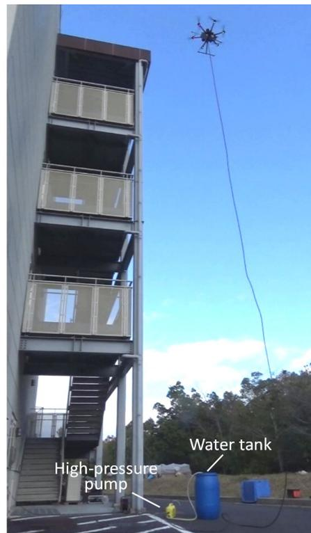
**Figure 14.** Pictures of the multirotor flying to maximum washable height. The height was about 12 m.
