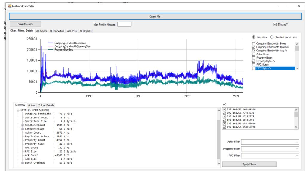
**Figure 10.** The Network Profiler interface for data analysis and transforming the file format.
