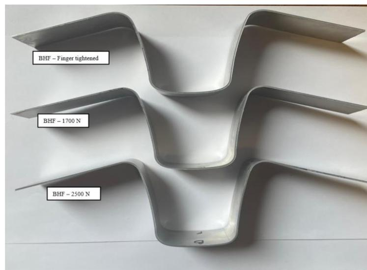
**Figure 25.** Profiles of Al/PP/Al specimens with 0.2/0.8/0.2 mm thickness combination after springback.
