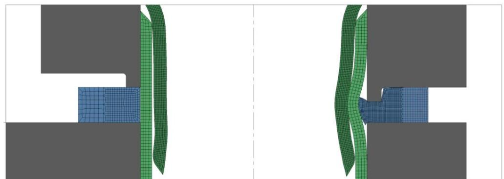
**Figure 3.** Detail of the finite element model after the upper tube reduction at the start of the sheet flange indentation (left) and at the end of the mechanical joining process (right). A mechanical connection between two PVC tubes by means of the aluminum sheet flange is depicted.
