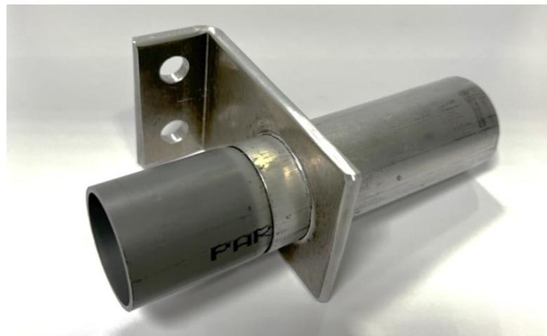
**Figure 12.** Example of PVC–Al tube connection produced by a sheet flange, having two holes for subsequent assembly.
