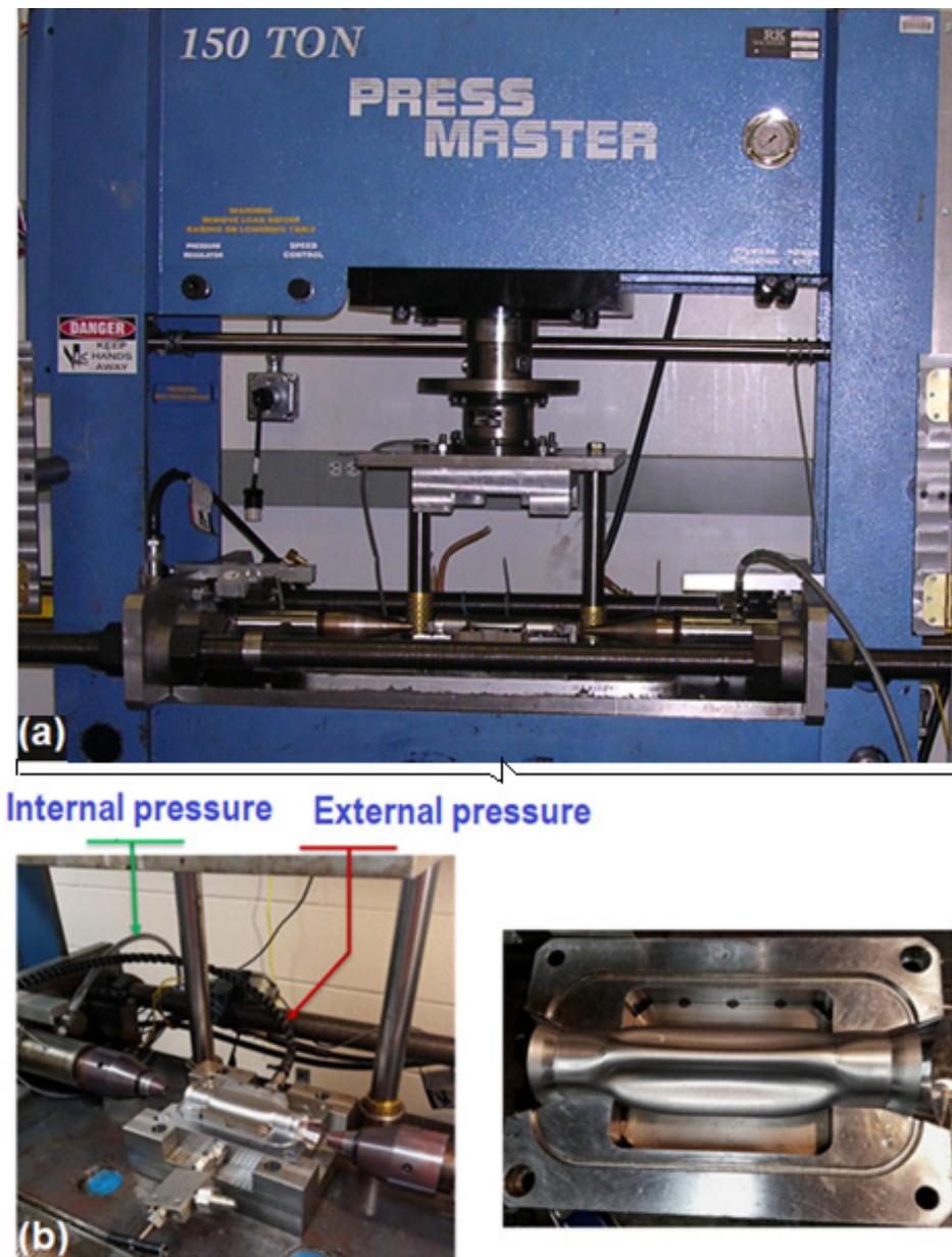
**Figure 6.** (a) A 150-ton hydraulic press, (b) dual-pressure THF tooling and a collapsed tubular blank.
