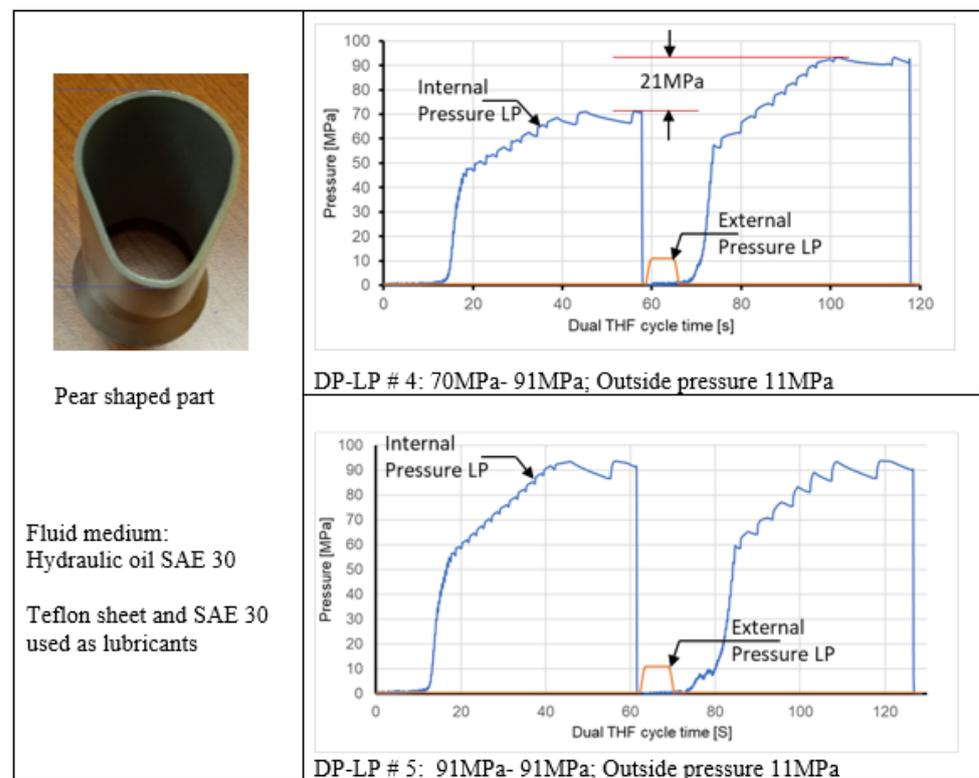
**Figure 8.** Loading paths used in dual-pressure THF for pear-shaped geometry.
