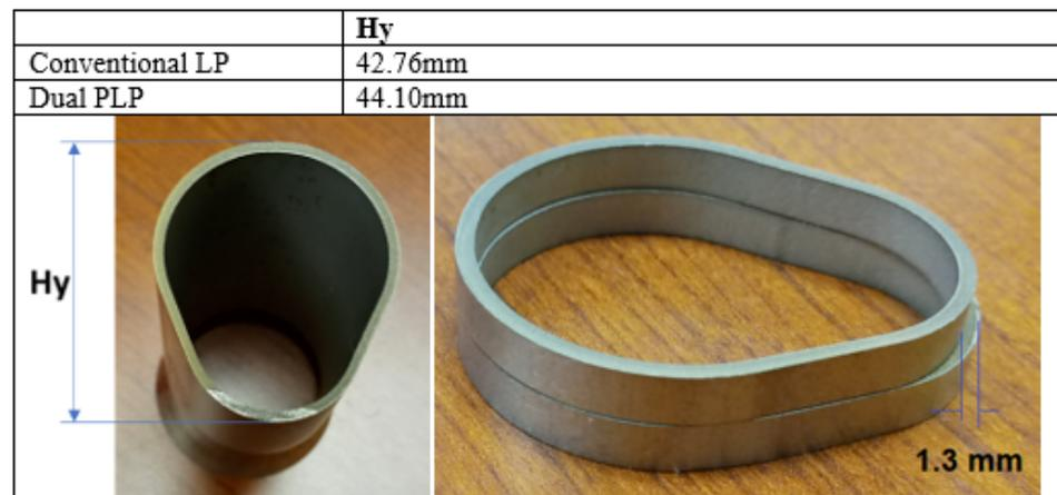
Figure 13. Load path # 4: 91 MPa, 11 MPa, and 91 MPa (pear shape using the oil SAE 30).
