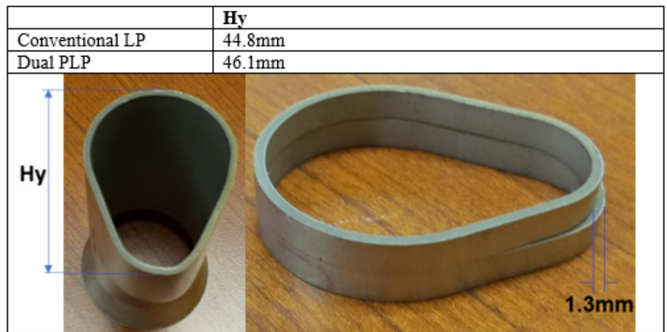
Figure 15. Load path #5: 91 MPa, 11 MPa, and 91 MPa (pear shape using Teflon sheet).
