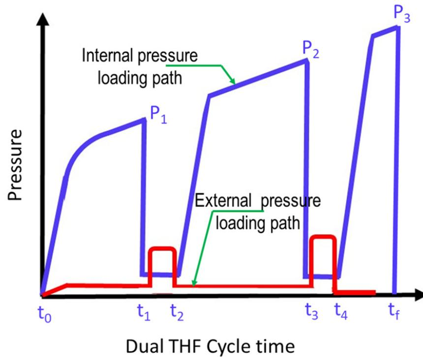
**Figure 3.** Hypothetical dual-pressure THF loading paths. “P1, P2, and P3 represent the maximum fluid pressure values reached during pressurization levels 1, 2, and 3, respectively”.
