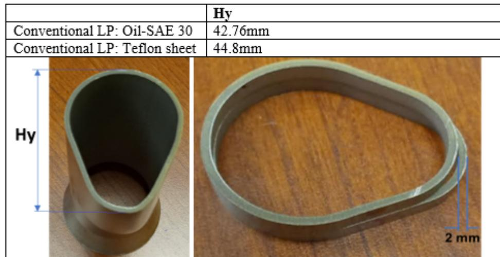
Figure 14. Influence on lubricant on protrusion height [ SAE 30 vs. Teflon sheet].
