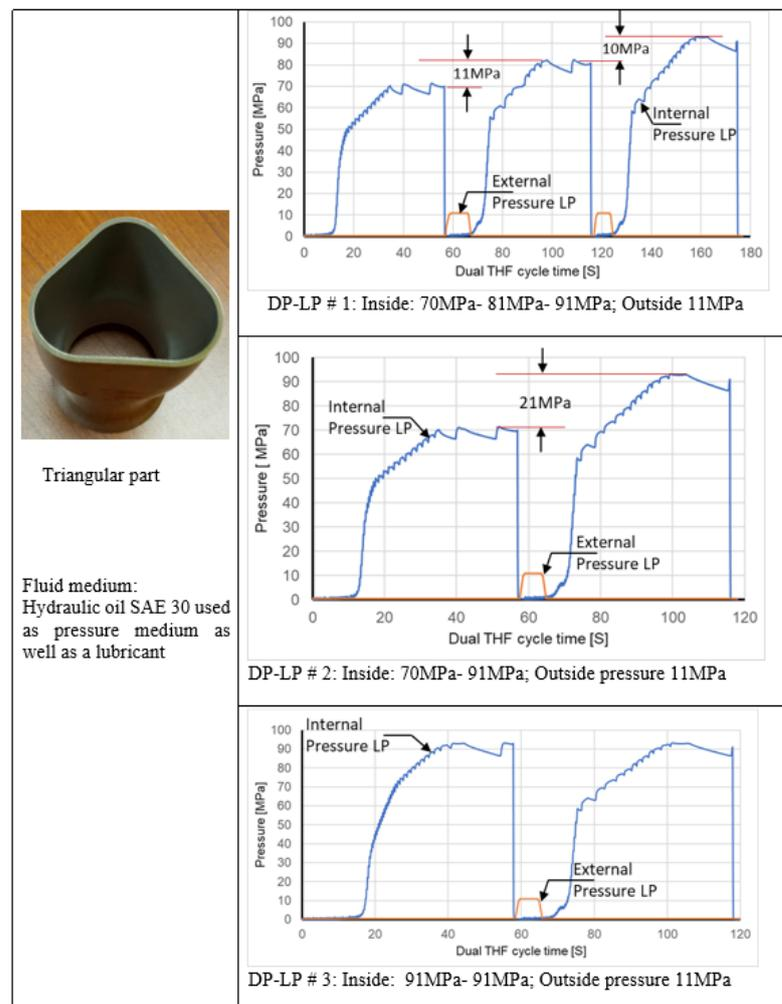
**Figure 7.** Loading paths used in dual-pressure THF for triangular parts.
