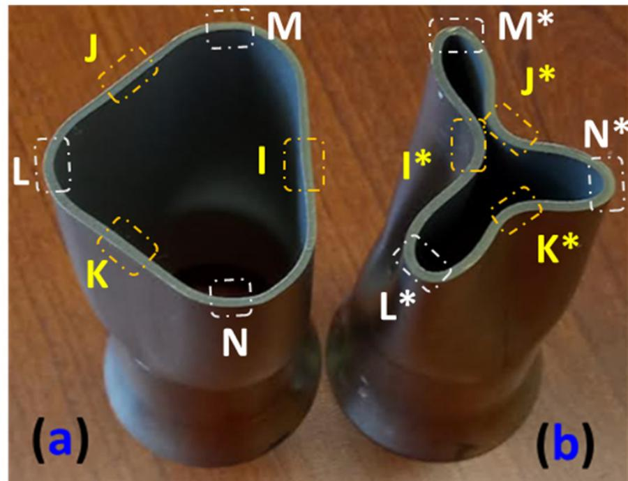
**Figure 11.** Plastic deformation during (a) internal and (b) external pressurization. The “\*” is used to differentiate between the deformation mode observed during external pressurization and the deformation mode exhibited during internal pressurization.
