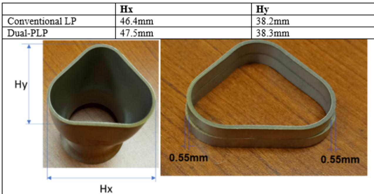
Figure 10. Dual-pressure LP#3: 91 MPa-11 MPa-91 MPa, comparison with CLP (triangular parts).
