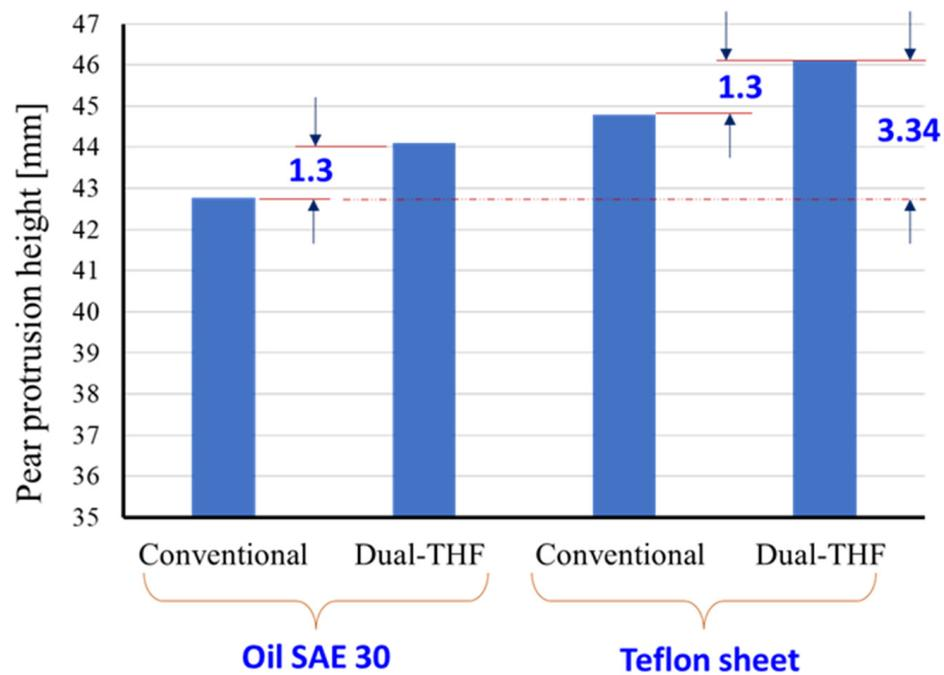
**Figure 16.** Influence of dual-pressure THF on formability for different lubrication conditions.
