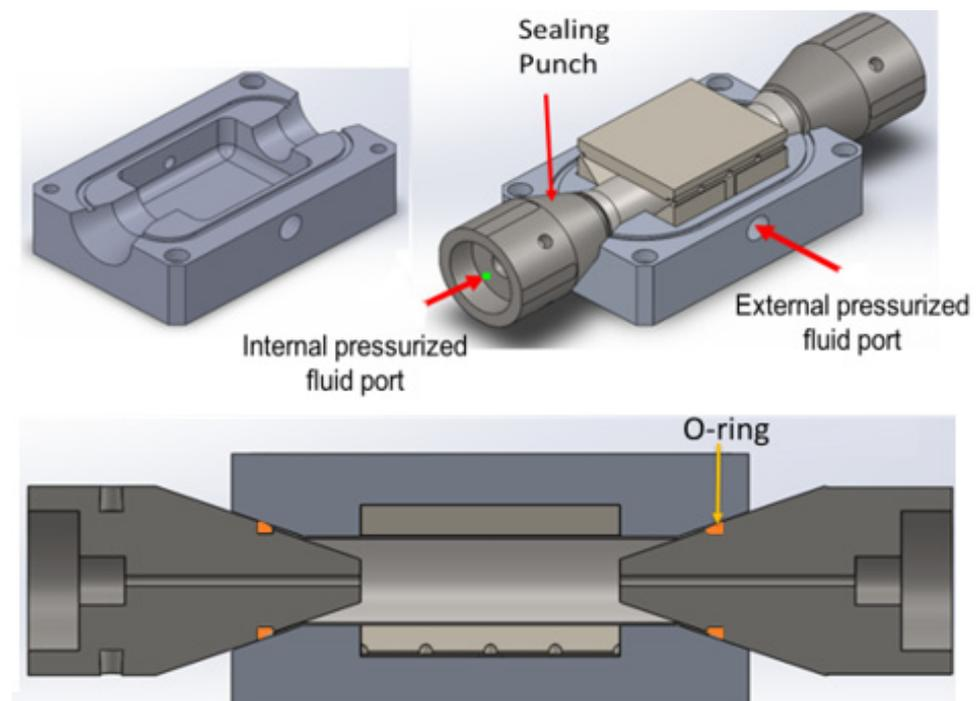
**Figure 5.** Tooling architecture for dual-pressure THF.
