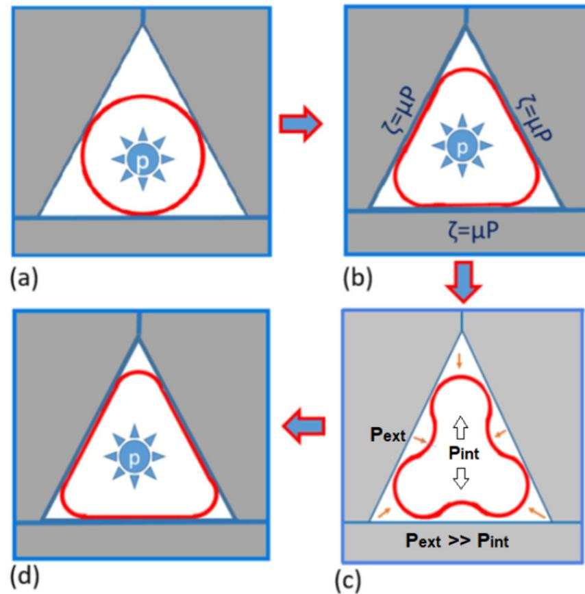
**Figure 2.** Dual-pressure tube hydroforming cycle: (a) Initial tube-die configuration before hydroforming, (b) deformed shape after 1st internal pressurization of the tube, (c) collapsed tube after external pressurization, and (d) 2nd level of internal pressurization to produce a part.
