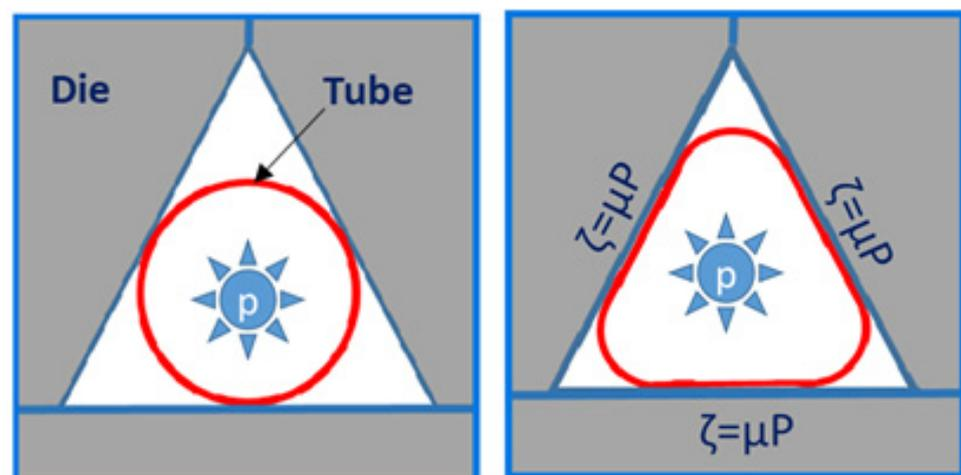
**Figure 1.** Conventional tube hydroforming.
