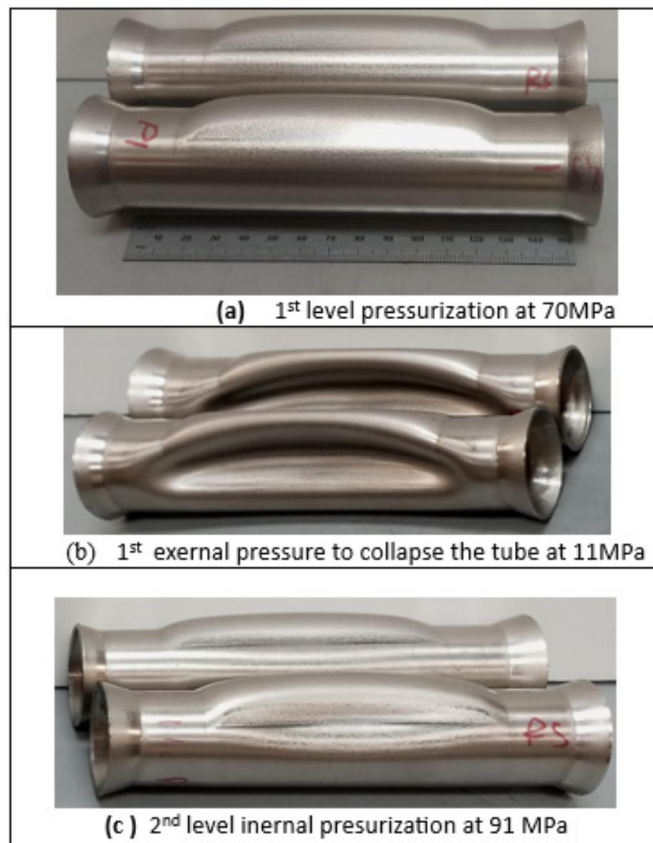
**Figure 12.** Dual-pressure LP# 4 for pear-shaped parts: (a) The tube deformation shape during the first level pressurization loading path at 70 MPa, (b) The tube deformation shape observed during external pressurization at 11 MPa, (c) The tube deformation shape for the second level pressurization loading path at 91 MPa.
