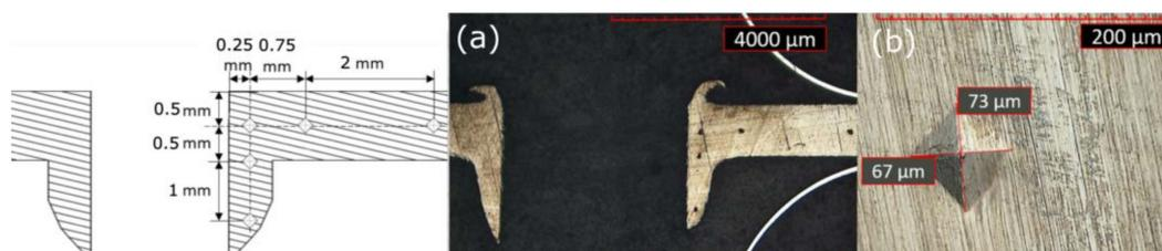
**Figure 5.** Cross-sectional hardness measurements: (a) locations of indents; (b) close-up of an indent.
