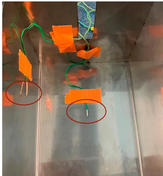
**Figure 4.** Sensors for measuring the temperature on the side and lid of the box.
