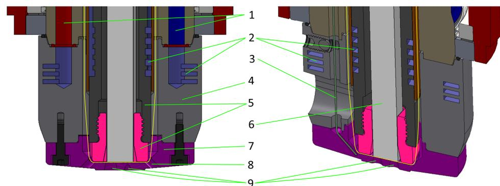
**Figure 1.** Cross-sections of AFED tooling: (1) coolant supply and return; (2) coolant passages; (3) thermocouple; (4) die holder; (5) guide tube with lower end (pink); (6) feedstock; (7) extrusion die; (8) outlet passages for material overflow to the sides; (9) extrusion channels. Note: all parts besides (5) and (6) rotate during the process (separation indicated by yellow line).
