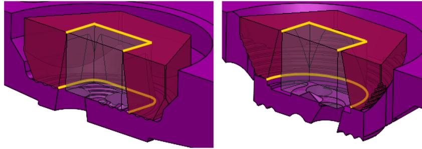
**Figure 7.** Initial (left) and revised (right) guide tube end/die interface. The initial design had a square taper, which allowed feedstock material to easily be forced between the die and guide tube end. The revised design had a transition from a square top to a circular bottom. Both contours of the taper (square and circular) are highlighted in yellow.
