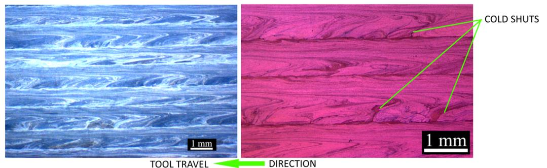
Figure 14. Left: Longitudinal overview along the traverse direction of the tool showing several deposited layers, coherence, and banded structures. Right: Longitudinal detail of the layers on the retreating side with magnification of the spacing and flaws. Tool travel direction is to the left.
