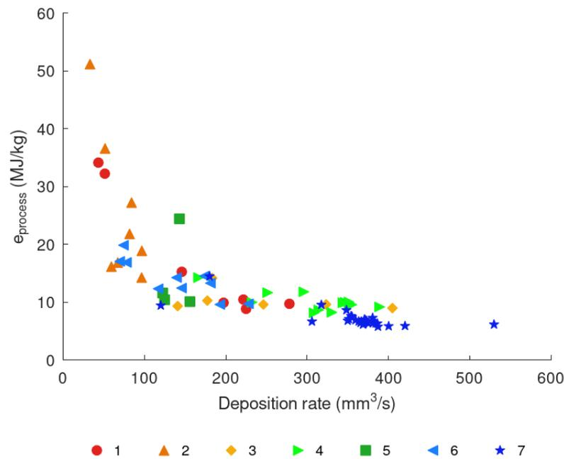
**Figure 8.** Specific process energy consumption (Equation (9)) by die number (see Figure 5) and volumetric deposition rate. The values are the averaged per deposition run during steady-state conditions.
