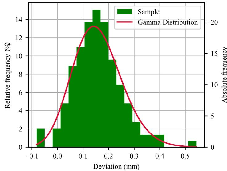
**Figure 5.** Example of fitting with a gamma distribution of the 150 measurements across the Y axis belonging to the 50–80 mm class.
