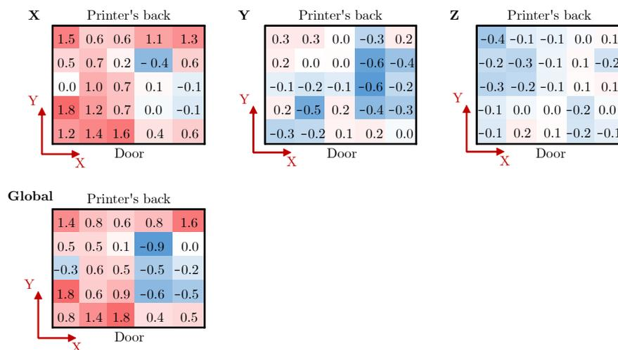
**Figure 10.** Average relative deviations in % depending on the X, Y, and Z axes and global indicator, blue is used for negative relative deviations, red for the positive, and white for the values approaching zero.
