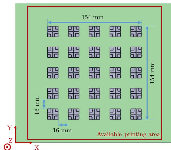
**Figure 2.** Distribution of the 25 COMPAQT parts on the build platform (in green) within the available printing area (red square).
