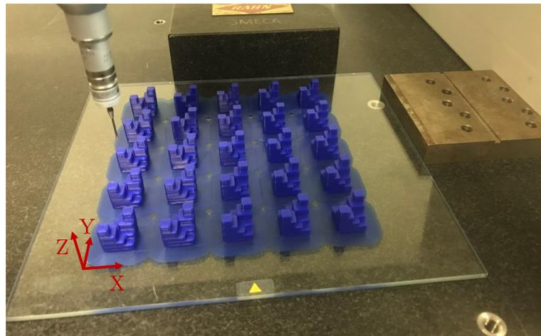
**Figure 4.** Measurement configuration used with the CMM.
