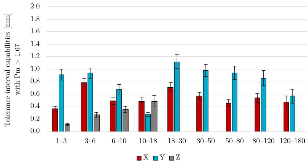
**Figure 8.** Potential tolerance interval capabilities in mm depending on the dimensional size ranges of ISO 286-1 considering a  $P_m$  target of 1.67 at a confidence level of 95%.
