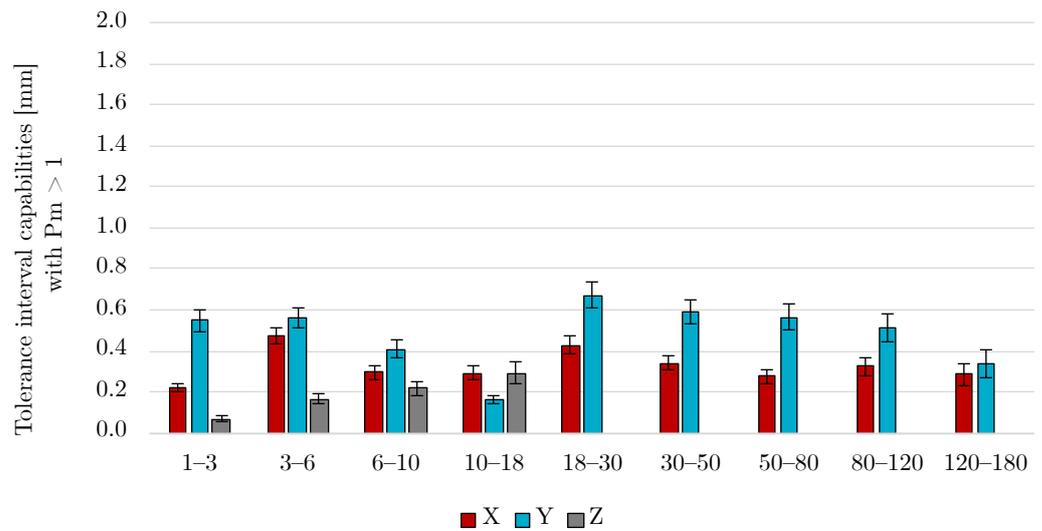
**Figure 9.** Potential tolerance interval capabilities in mm depending on the dimensional size ranges of ISO 286-1 considering a  $P_m$  target of 1 at a confidence level of 95%.
