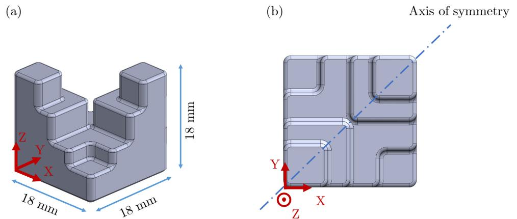
Figure 1. Design of the COMPAQT part with maximal dimensions (a) and axis of symmetry (b).
