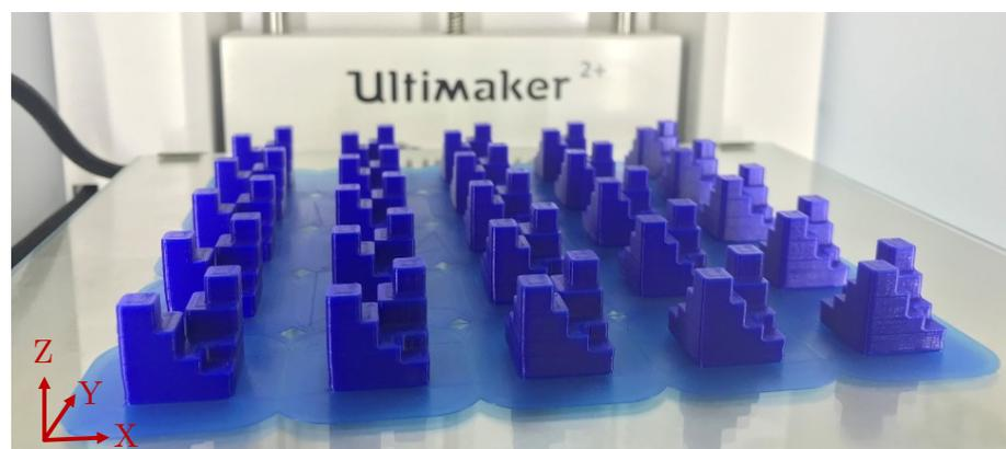
**Figure 3.** Batch of 25 COMPAQT parts after their manufacturing in an Ultimaker 2+ printer.
