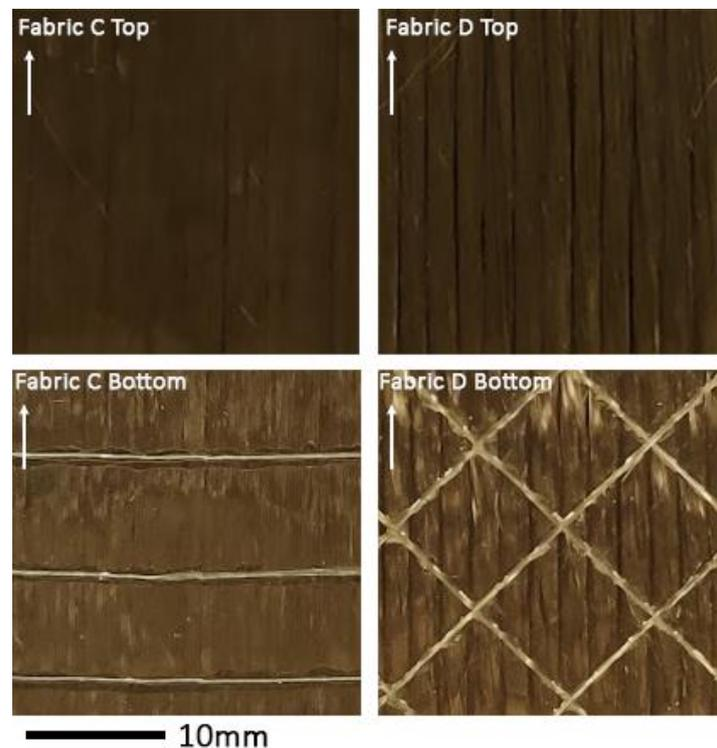
**Figure 2.** Top and bottom views of the two distinct types of fabrics. Fiber direction is indicated with arrows.
