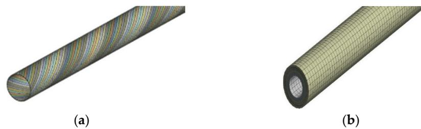
**Figure 4.** Mesh of flexible riser model. (a) Tensile armor layer, (b) Overall model
