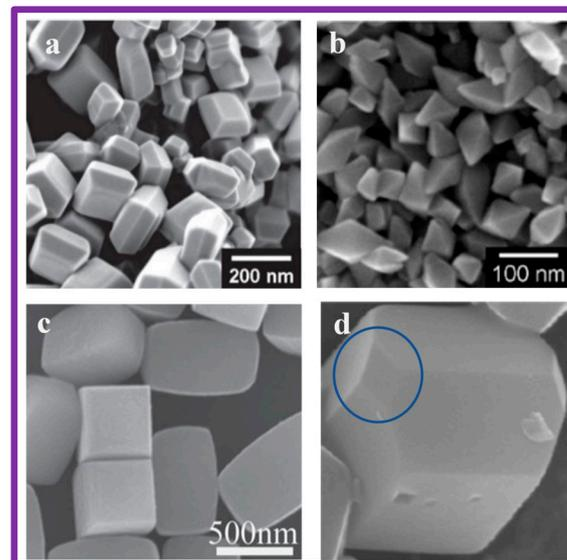
**Figure 9.** SEM images of crystals exposing different facets: (a) square  $\{001\}$  and trapezoidal  $\{101\}$  facets [39]; (b) triangular  $\{101\}$  facets in perfectly octahedral crystals [40]; (c) square  $\{001\}$  and rectangular  $\{100\}$  facets [37]; (d) square  $\{001\}$ , trapezoidal  $\{101\}$  and rhombus-shaped  $\{110\}$  facets [41]. Reprinted with permission from ref. [37,39–41].
