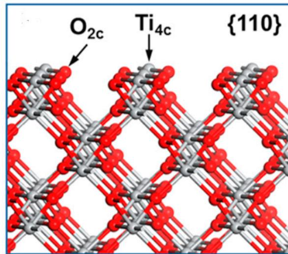
**Figure 11.** Surface atomic structures of the {110} crystal facet [10]. Reprinted with permission from ref. [10].
