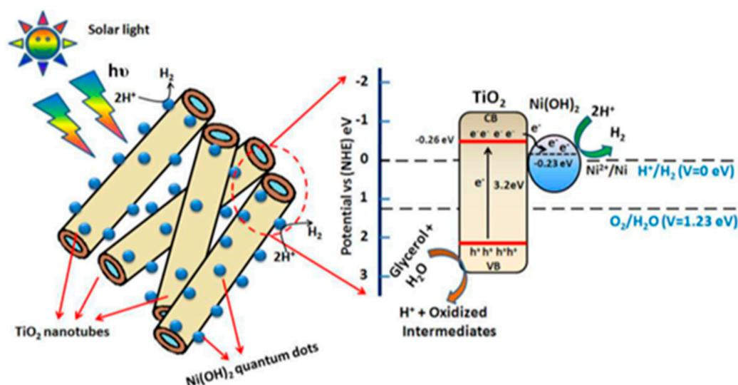
**Figure 4.** The mechanism for H<sub>2</sub> evolution on Ni(OH)<sub>2</sub>/TiO<sub>2</sub> nanotubes [28]. Reprinted with permission from ref. [28]. Copyright 2020 American Chemical Society.
