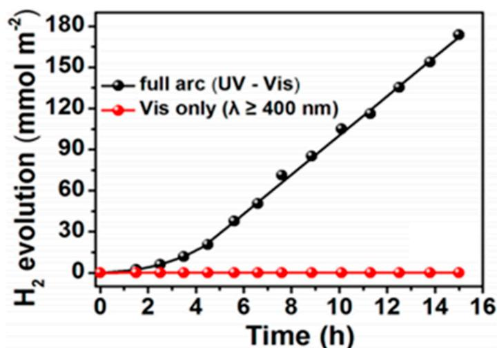
**Figure 13.** Time course of H<sub>2</sub> generation from a methanol solution with a catalyst developed by Hu et al. [10] Reprinted with permission from ref. [10].
