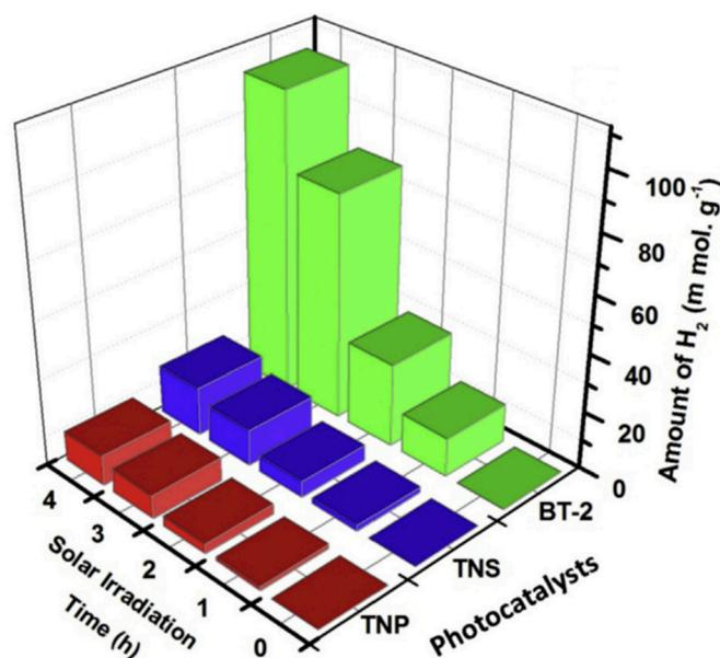
**Figure 5.** Solar photocatalytic activity comparison of  $\text{TiO}_2$  P-25 nanoparticles (TNP), a non-modified  $\text{TiO}_2$  nanostructure (TNS) and the  $\text{Bi}_2\text{O}_3$ -modified nanostructure (BT-2) [29]. Reprinted with permission from ref. [29]. Copyright 2017 Elsevier.
