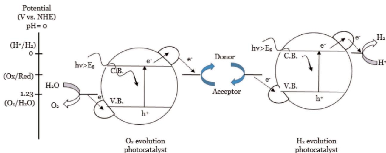
**Figure 14.** Schematic diagram for photocatalytic water splitting using a Z-scheme photocatalytic system [2]. Reprinted with permission from ref. [2].
