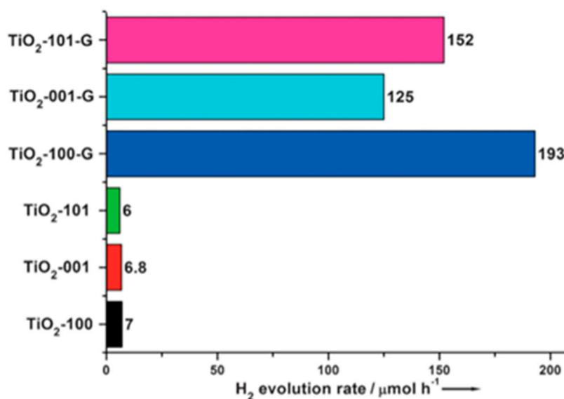
**Figure 10.** H<sub>2</sub> evolution rates from a methanol solution catalyzed by TiO<sub>2</sub> nanocrystals and TiO<sub>2</sub>-graphene nanocomposites [38]. Reprinted with permission from ref. [38].
