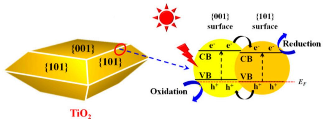
**Figure 12.** Mechanism of the surface heterojunction [46]. Reprinted with permission from ref. [46].
