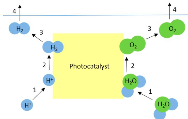
**Figure 3.** Schematic representation of mass transfer steps in photocatalytic water splitting. (1) Adsorption of the reactants, (2) reduction/oxidation of the reactants, (3) desorption of the products, and (4) transfer of the products from the photocatalyst surface to the gas phase.
