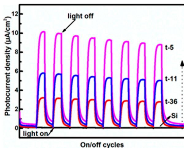
**Figure 7.** Photocurrent response (0.4 V bias) of selected catalysts and Si substrate electrodes in  $1 \text{ mol}\cdot\text{L}^{-1} \text{ Na}_2\text{SO}_4$  under visible-light illumination and in dark where t-5, t-11, and t-36 represents catalysts with an average film thickness of 0.28, 0.79, and 2.26  $\mu\text{m}$ , respectively [9]. Reprinted with permission from ref. [9].
