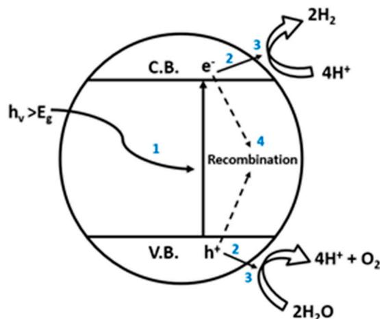
**Figure 2.** Schematic representation of photocatalytic water splitting with (1) light absorption and charge excitation from the valence band to the conduction band, (2) the transfer of the photogenerated electrons and holes to the catalyst surface, (3) surface redox reactions, and (4) a charge recombination. (VB valence band, CB: conductance band, and TR: trapped).
