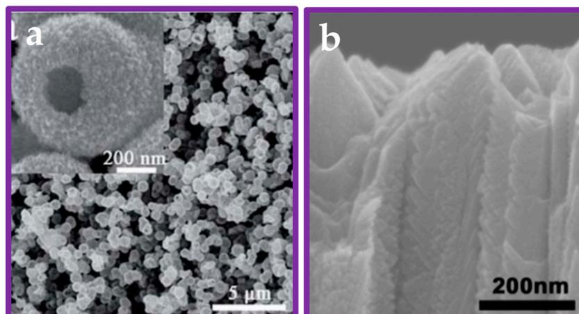
**Figure 6.** (a) SEM images of the stable mesoporous black TiO<sub>2</sub> hollow spheres [30]. Reprinted with permission from ref. [30]. (b). Lateral view of high-resolution SEM images of the TiO<sub>2</sub> catalyst prepared [9]. Reprinted with permission from ref. [9].
