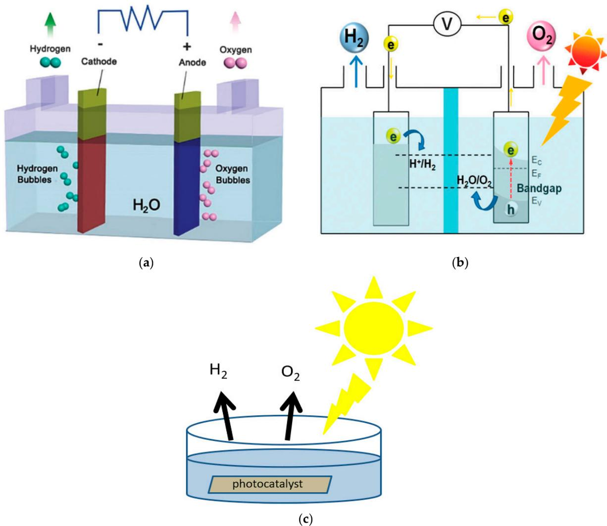
**Figure 1.** Processes of (a) water electrolysis [1] (reprinted with permission from ref. [1]), (b) photo-electrochemical water splitting [8] (reprinted with permission from ref. [8]), and (c) photocatalytic water splitting.
