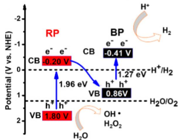
**Figure 16.** Schematic illustration of direct Z-scheme charge transfer pathway [60]. Reprinted with permission from ref. [60].
