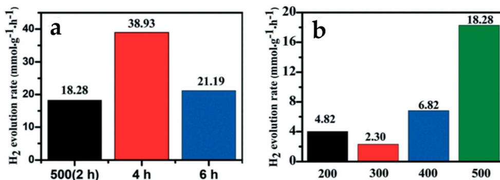
**Figure 18.** (a) Comparison of hydrogen evolution rates for Zn<sub>0.67</sub>Cd<sub>0.33</sub>S solid-solution nanosheets with a varying sulfurization temperature [62]. Reprinted with permission from ref. [62]. (b) The comparison of the hydrogen evolution rates for ZnO/Zn<sub>x</sub>Cd<sub>1-x</sub>S for varying oxidation times [62]. Reprinted with permission from ref. [62].
