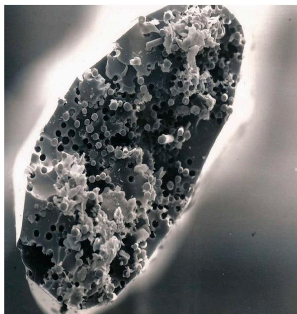
**Figure 5.** Micrograph showing a typical fracture surface of the minicomposite test specimen. Scale unit: 100 microns.
