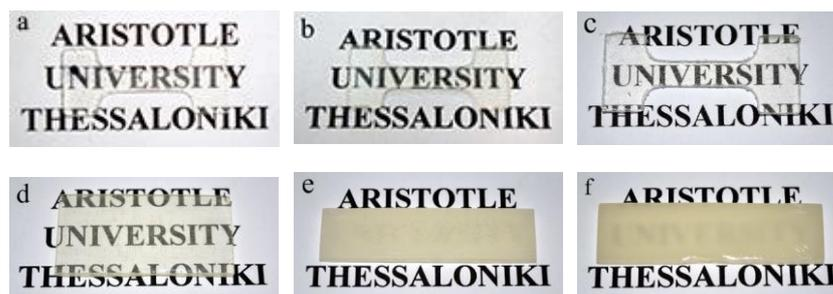
**Figure 3.** Selected photographs of SBA-15 mesocomposites: (a) pristine rubbery, (b) rubbery/9% SBA-15 (10), (c) rubbery/3% SBA-15-propyl, (d) pristine glassy, (e) glassy/3% SBA-15 (5), and (f) glassy/3% SBA-15-amino.
