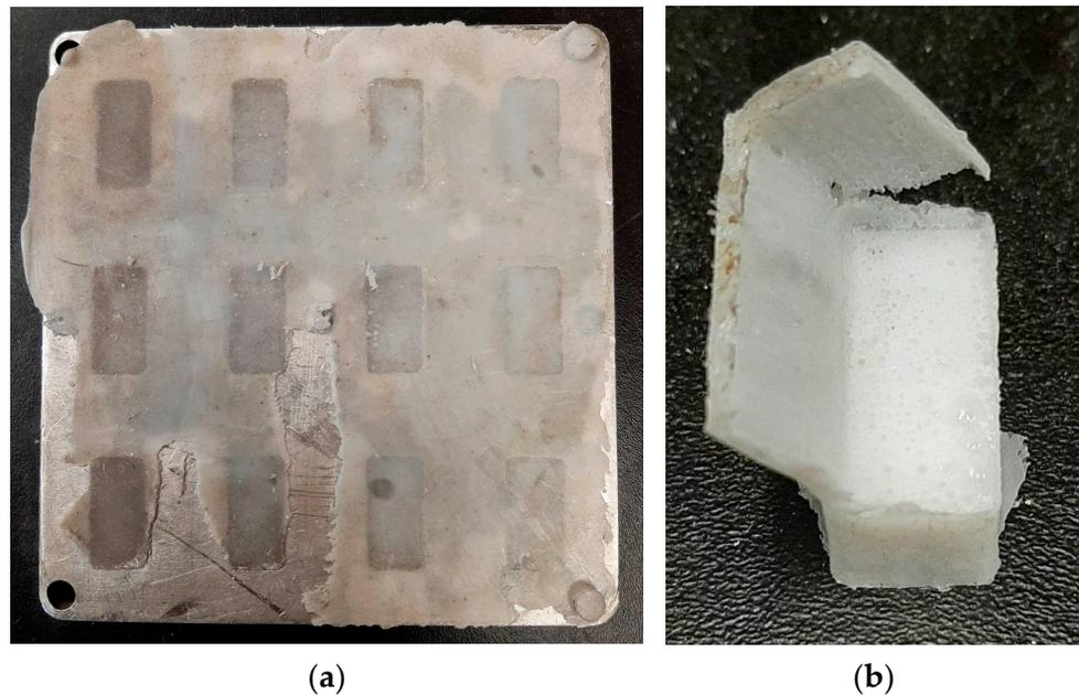
**Figure 6.** (a) Released mold with visible flash. Mold was filled with 50% sand on the left and 20% sand on the right. (b) The 100% PC sample example immediately following part ejection and prior to cleanup.
