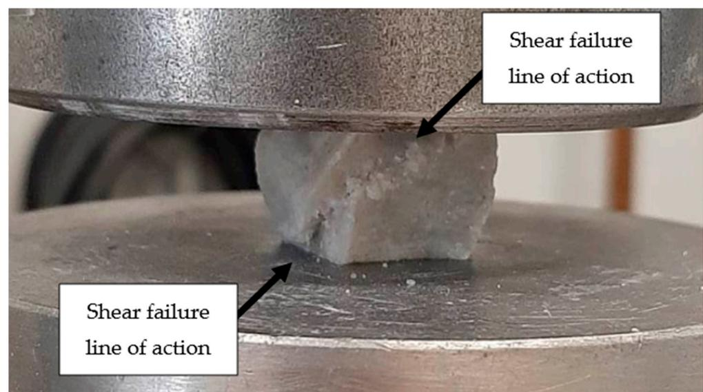
**Figure 11.** Shear failure of the 50% sand sample during compression testing.
