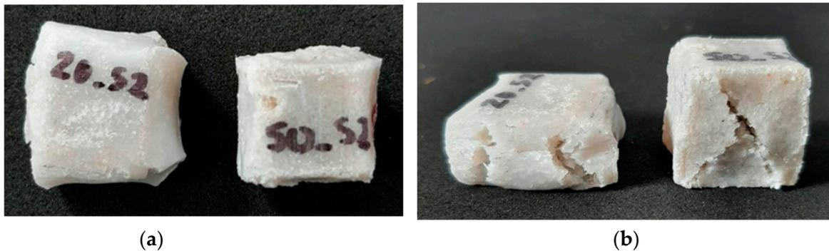
**Figure 10.** Deformed sample differences between high and low sand compositions. (a) Top view of the 20% sand (left) and 50% sand (right) samples demonstrating the increase in deformation contributing to larger cross-sections in lower sand compositions. (b) Side view of the 20% sand (left) and 50% sand (right) samples indicating higher strain associated with thermoplastic flow in lower sand compositions.
