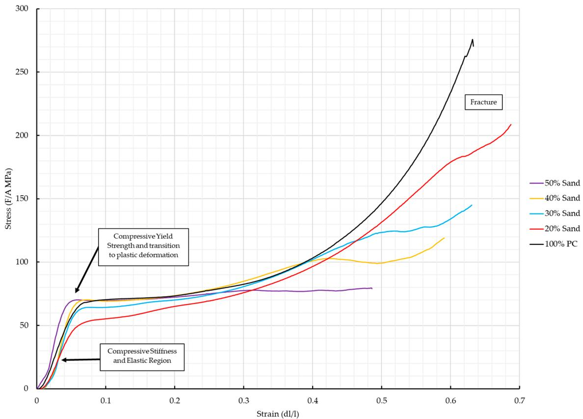
**Figure 8.** Stress vs. strain across a range of sand/PC compositions by weight compared to the optimal 100% PC control. The datasets shown are representative samples of the different compositions.
