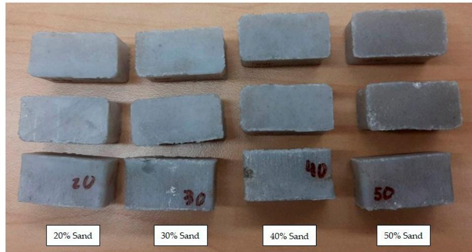
**Figure 7.** Plastic sand bricks matrix of samples. Columns are identified from left to right as 20%, 30%, 40%, and 50% sand-to-plastic ratios by weight.
