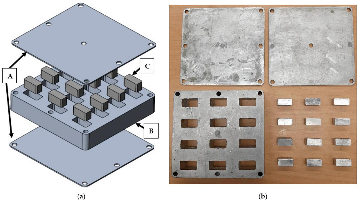
**Figure 2.** Laser-cut aluminum mold components and alignment orientation. (a) 3-D render and (b) physical components of (A) Mold Lid X2, (B) ASTM D695 Pocket Mold, (C) Mold Plug X12.
