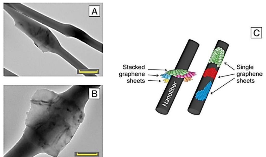
**Figure 6.** TEM micrographs of nanofibrous mats with (A) 5 wt.% graphene (scale bar: 500 nm); (B) 15 wt.% graphene (scale bar: 300 nm); and (C) sketch of graphene disposition along the nanofiber surface. TEM = Transmission electron microscopy. Reprinted with permission from [84]. 2019, Elsevier.
