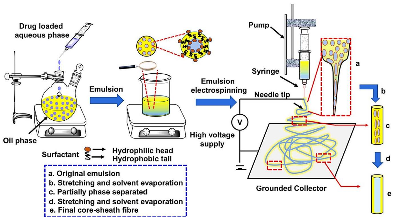
**Figure 4.** Flowchart of emulsion electrospinning setup and process. Reprinted with permission from [4]. 2022, MDPI.
