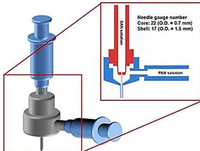
**Figure 1.** Graphic of a syringe needle system for coaxial electrospinning. O.D. = outer diameter; SAN = poly(styrene-co-acrylonitrile); PAN = poly(acrylonitrile). Reprinted with permission from [58], 2012, Springer.
