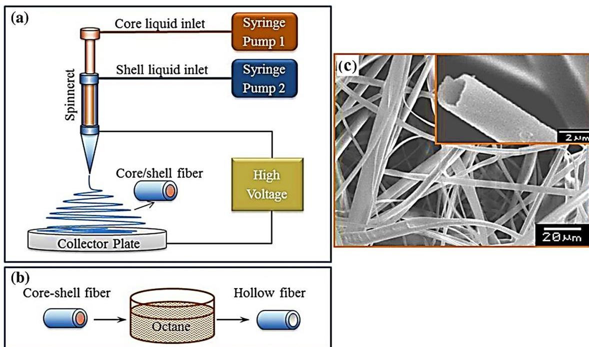
Figure 3. Core-shell fiber formation: (a) schematic of coaxial electrospinning setup; (b) diagram of fiber core extraction; and (c) fiber size distributions of solid electrospun and hollow fibers. Reprinted with permission from [59]. 2015, Springer.
