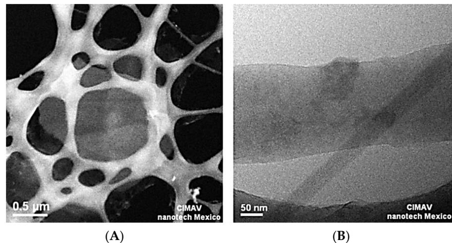
**Figure 5.** STEM images showing (A) few layers of GOFT platelet (less than 4), and (B) nanocomposite nanofiber containing a thicker GO platelet. STEM = Scanning transmission electron microscopy; GOFT = nitroxide-functionalized graphene oxide layers; GO = graphene oxide. Reprinted with permission from [83]. 2014, Elsevier.
