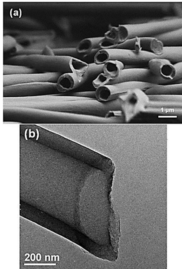
Figure 2. (a) Field emission scanning electron microscopy and (b) transmission electron microscopy images of a hollow electrospun carbon nanofiber. Reprinted with permission from [58]. 2012, Springer.
