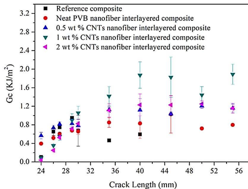
**Figure 8.** Mean fracture energies,  $G_c$ , with respect to crack length of reference and interlayered composites. PVB = pol(vinyl butyral); CNTs = carbon nanotubes. Reprinted with permission from [98]. 2018, Elsevier.
