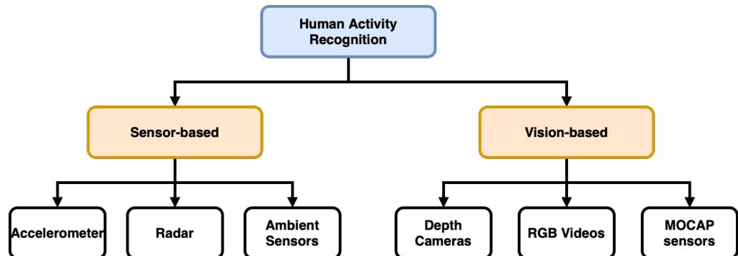
**Figure 6.** A general hierarchy of HAR methods. Typically, HAR is separated in sensor-based and vision-based approaches. The two major subcategories are divided into their respective sensors that are leveraged.
