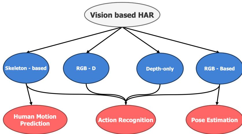
**Figure 9.** Typically used modalities in vision-based methods in HAR. Due to the wide range of applications of HAR, vision-based methods can be further categorized in subsequent tasks. Most notable are human motion prediction, action recognition and pose estimation.
