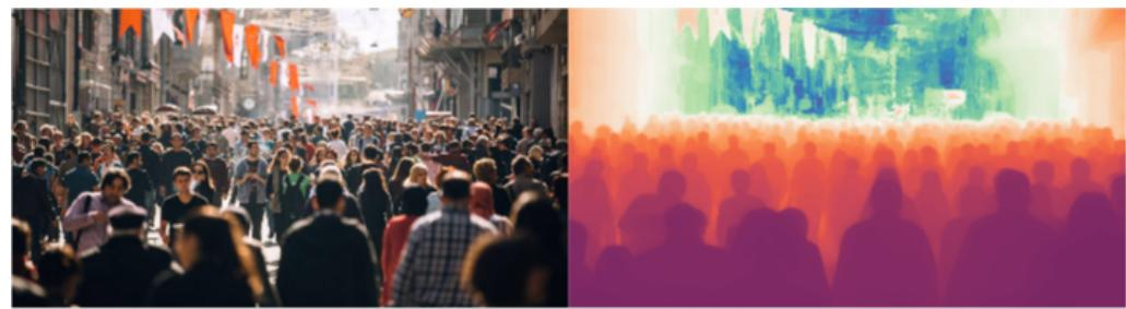
**Figure 7.** An example of an RGB-D image. The source RGB image appears to the left and its corresponding depth map to the right. Objects that appear closer have a darker red color while the furthest objects appear blue. A notable dataset that is available for HAR problems and provides both RGB and LiDAR scanned depth maps is the Human4D dataset [40].
