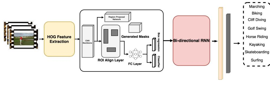
**Figure 10.** The framework proposed in [97]. First, the video is split into a sequence of RGB images and consequently fed into an instance segmentation module, typically a MaskRCNN [96]. The per-frame semantic representation extracted from the segmentation module are then processed by an RNN, before they are fed to a fully connected layer to finally infer the activity class.
